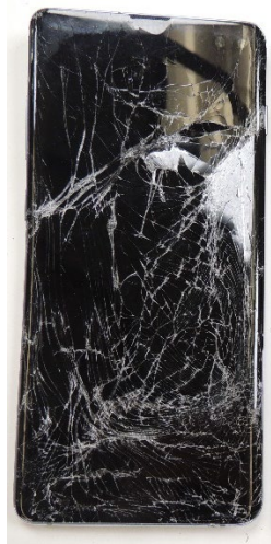
Figures 7. Damaged Samsung Galaxy S10 as received.
