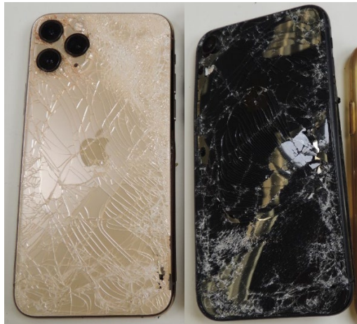
Figures 3 & 4. Damaged iPhone 11 Pro (left) and iPhone XR (right) as received.
