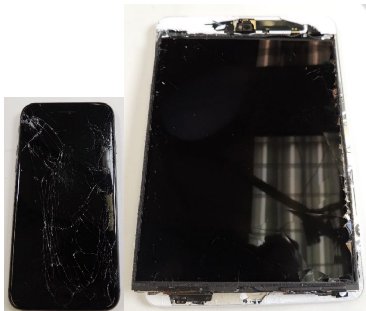
Figures 5 & 6. Damaged iPhone 8 (left) and iPad Mini 2 (right) as received.
