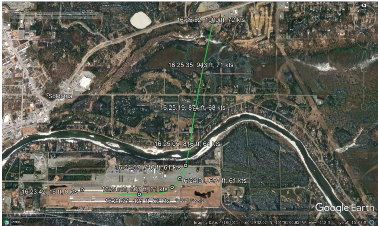
Figure 10. Data extracted from the Garmin GDU 460 memory chip.
