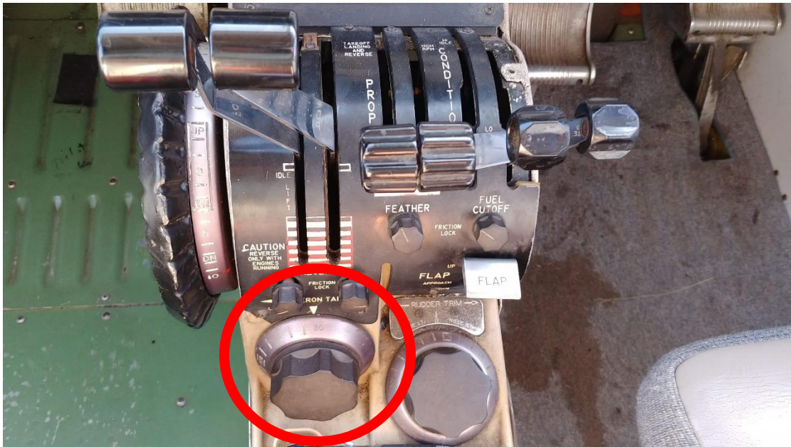
Photo 8: Photo of N256TA Aileron trim, indicated by red circle. Photo shows aileron trim knob indicating full left wing down orientation. 119
