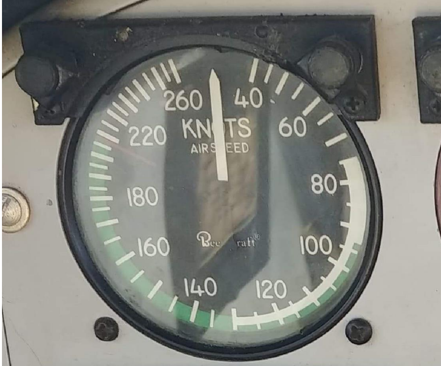
Photo 9: Close-up photo taken by a former Oahu Parachute Center pilot, showing the airspeed indicator on the accident airplane.
