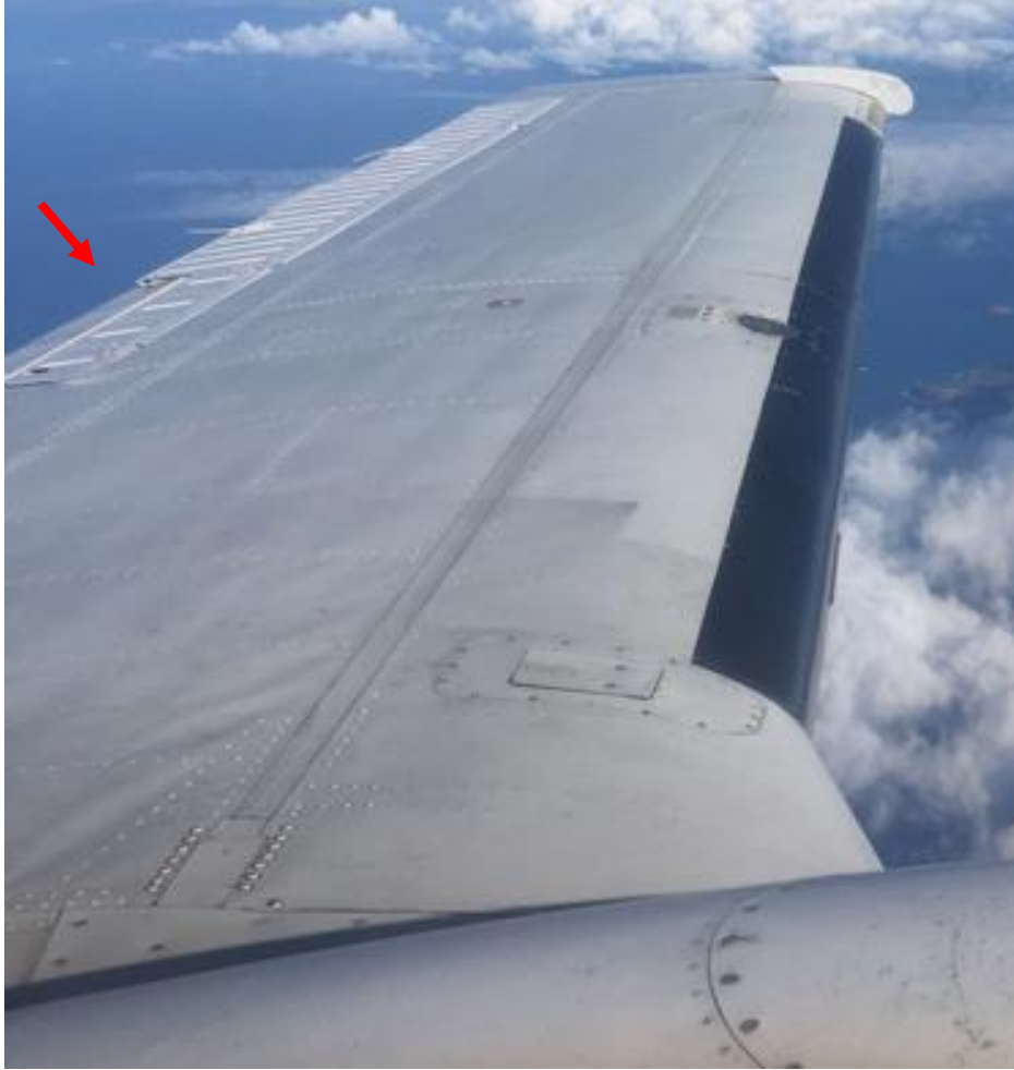
Photo 4: Inflight photo of N256TA during 2017 delivery to Hawaii. The red arrow shows the aileron trim tab deflection. 118
