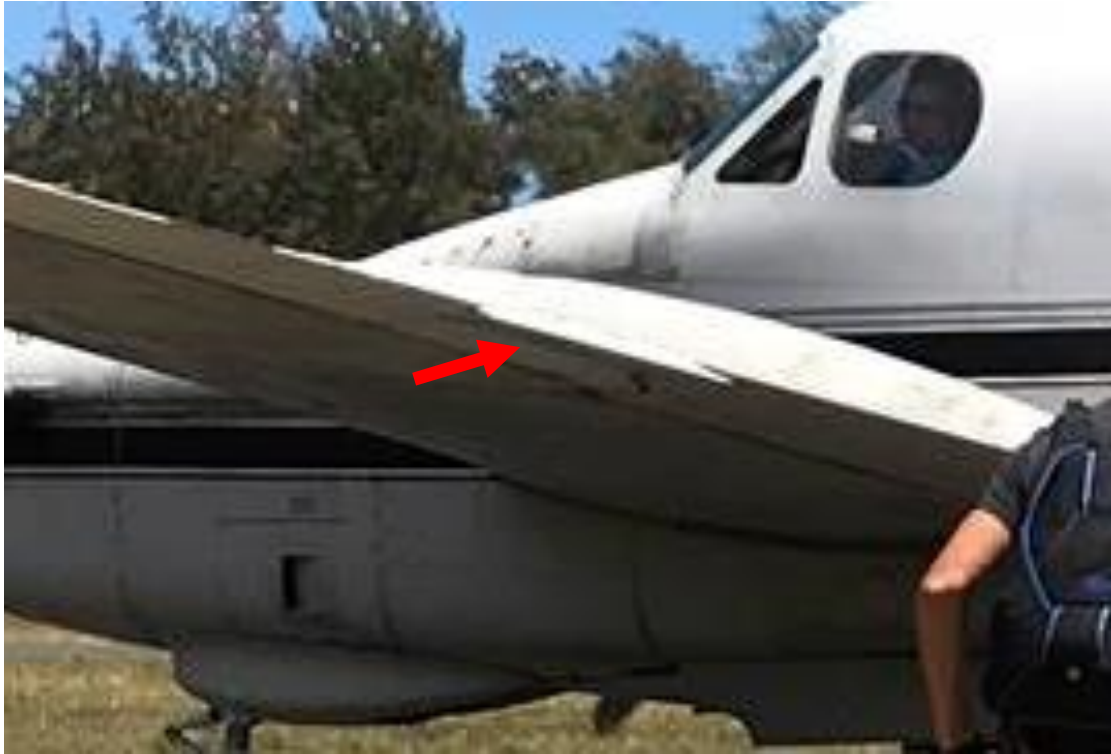
Photo 7: Enlargement of previous photo showing aileron trim tab in a trailing edge down position, indicated by the red arrow.
