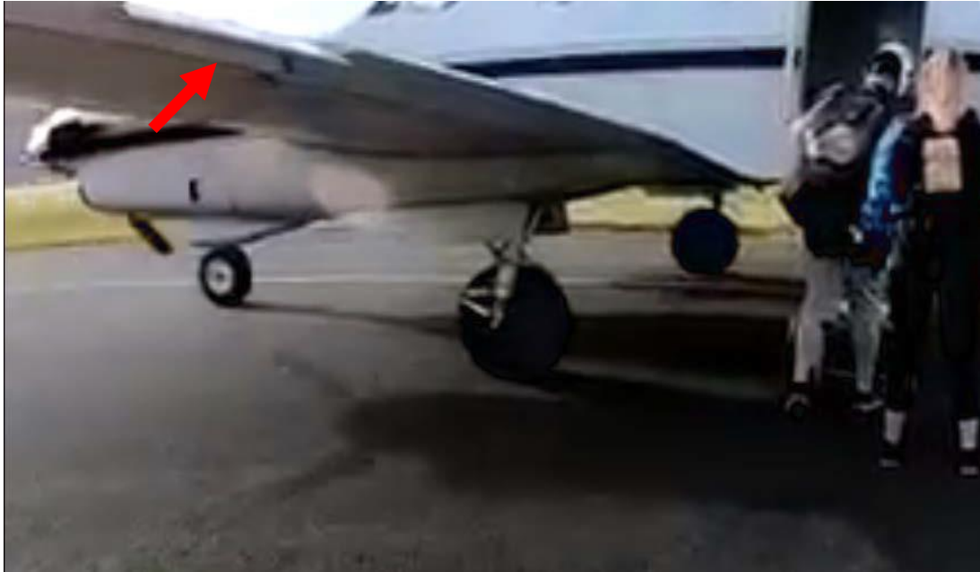
Photo 5: Witness-provided photo of N256TA at HDH showing aileron trim tab in a trailing edge down position, indicated by the red arrow. Date of photo is unknown.
