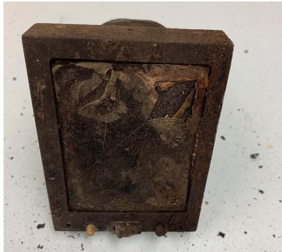
Figure 1. Damaged exterior of EDM.
