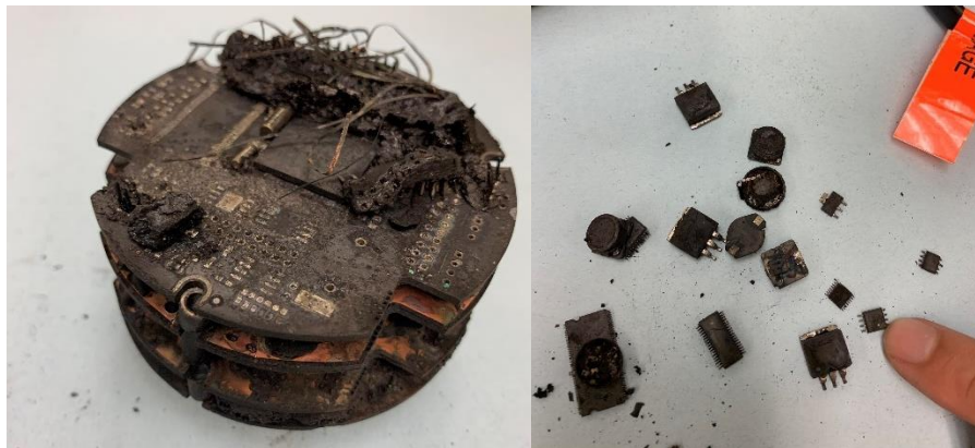
Figure 2. Damaged internal components of EDM (left) and displaced memory chips from device (right). The specialist's finger is pointing to the NVM chip containing flight data.
