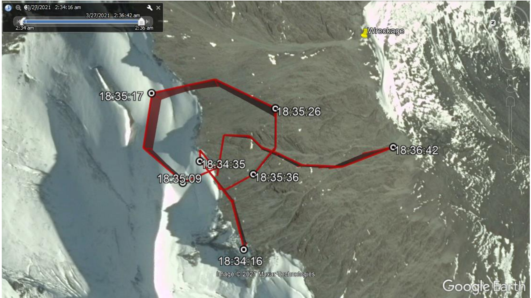
Figure 14. A top down view of the final tracklog points for the accident leg. Previous portions of the accident leg have been removed for clarity. The final resting place of the wreckage is depicted as a yellow pin.
