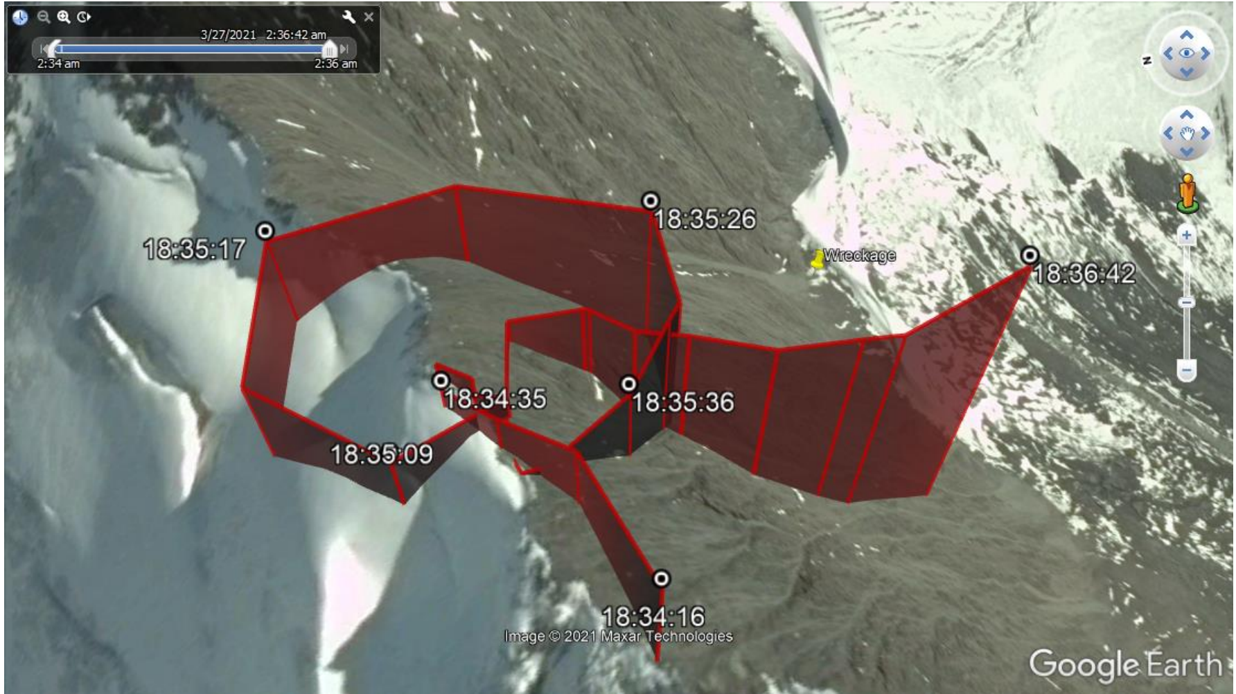
Figure 13. An askew view of the final tracklog points for the accident leg. Previous portions of the accident leg have been removed for clarity. The final resting place of the wreckage is depicted as a yellow pin.
