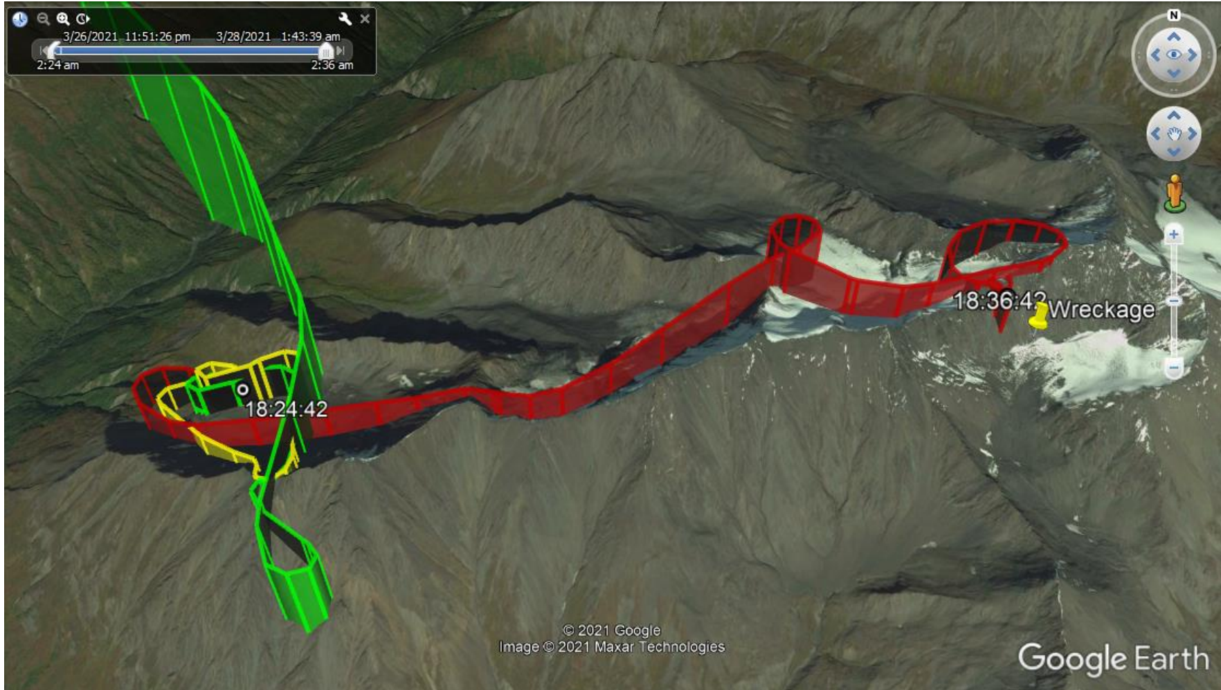
Figure 11. A overview of the helicopter's GPS tracks for the accident leg (shown in red). The start and end time of the data is shown. The final resting place of the wreckage is depicted as a yellow pin.
