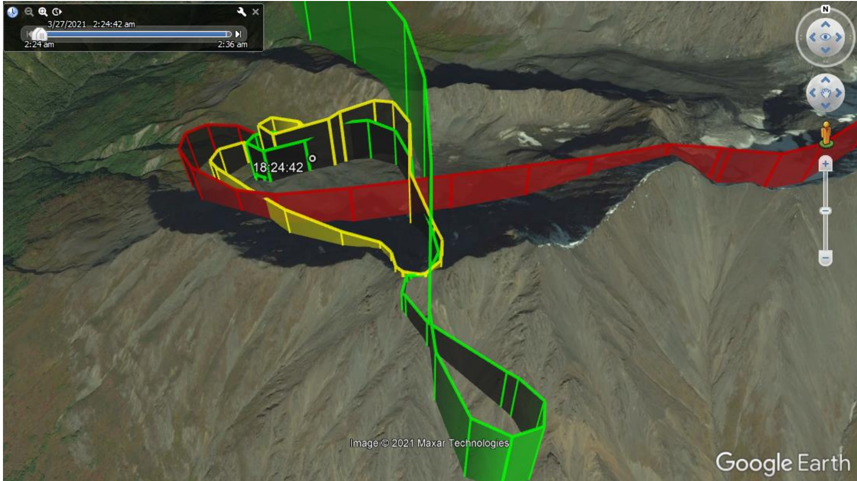
Figure 10. A depiction of the GPS tracks for the helicopter's departure on the 4 th and final (accident) leg. The accident leg is shown in red. Data recording for this leg began at 18:24:42.
