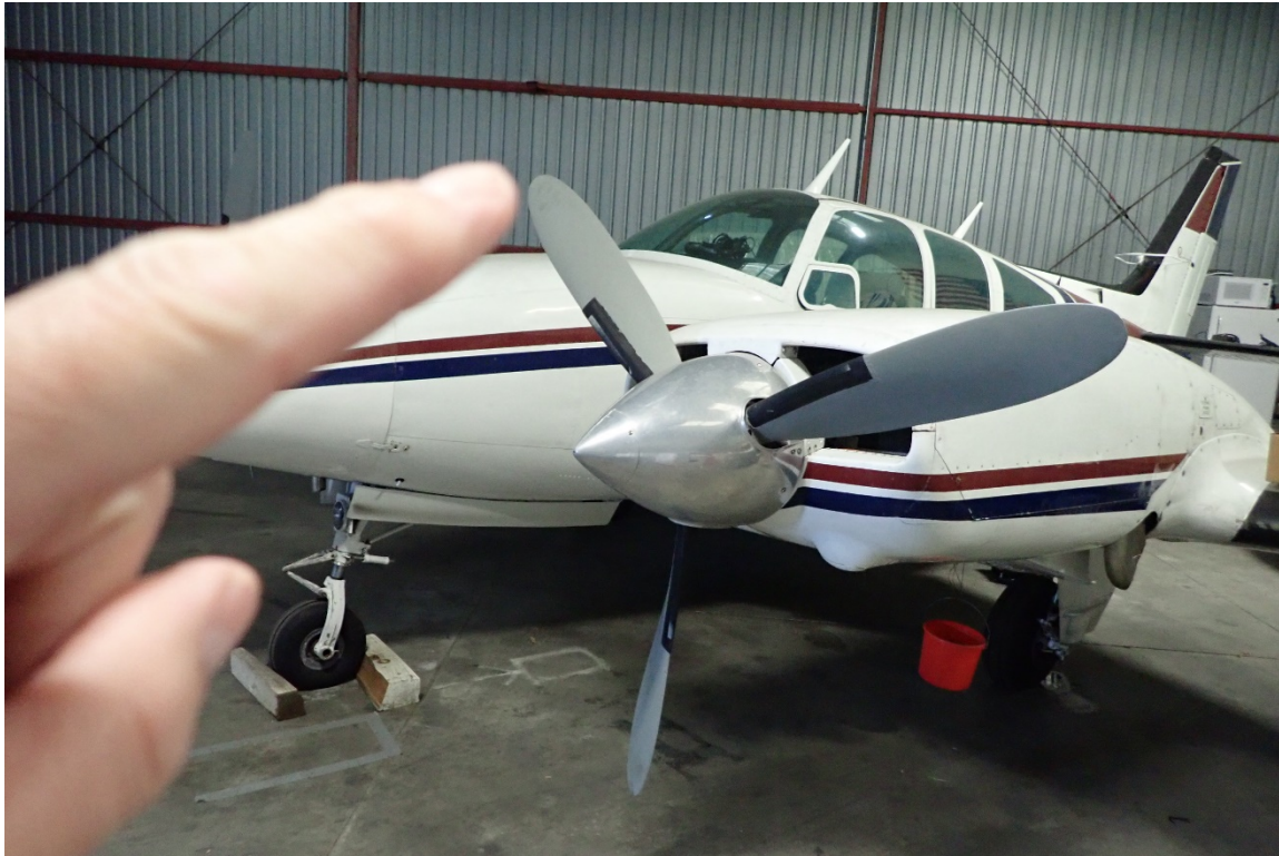
Photo 1 – Baron, with Finger indicating Contact Area with M65MY Elevator
