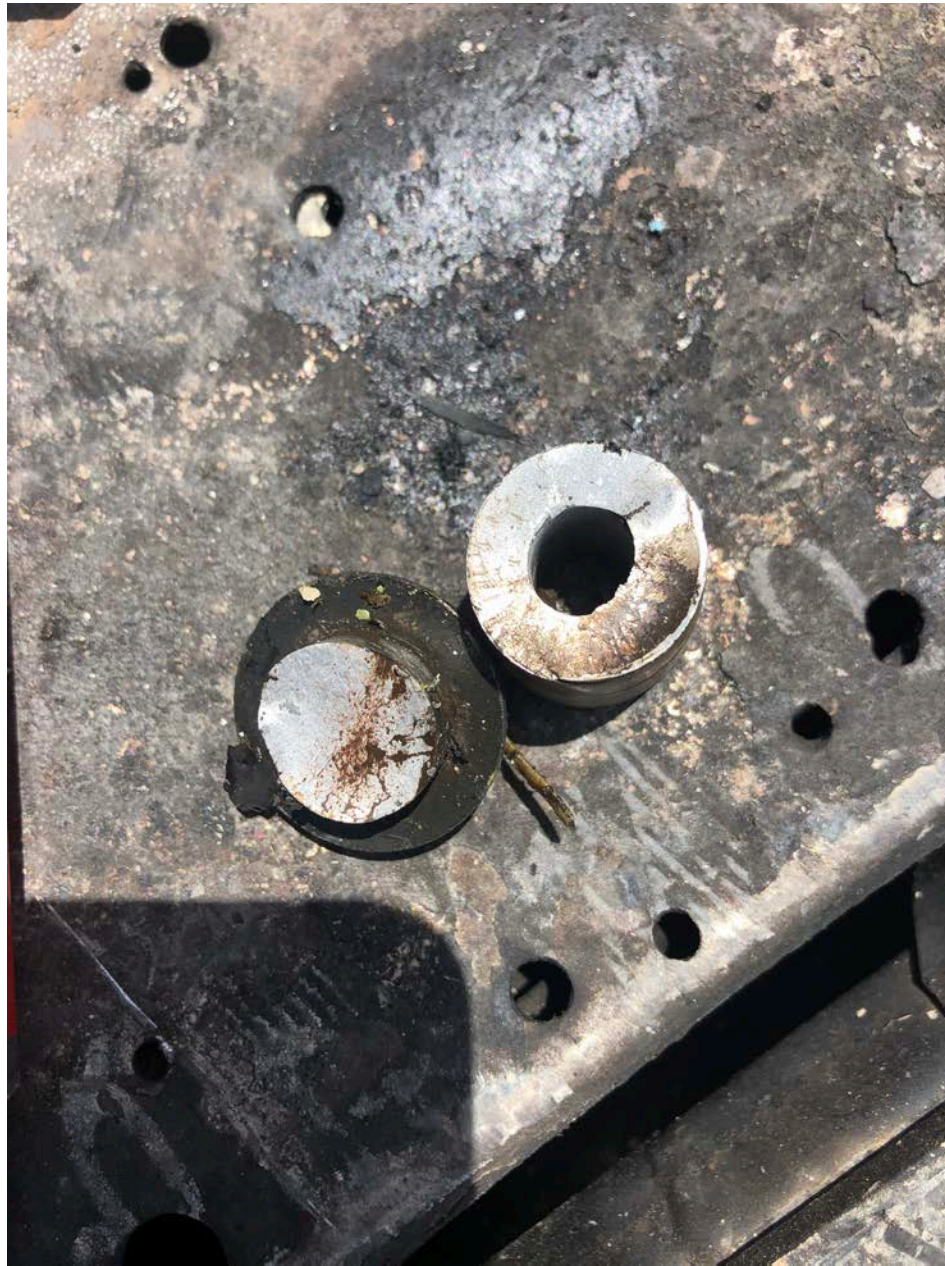
Photo 11 – Outboard portions of the tailwheel locking pin.
