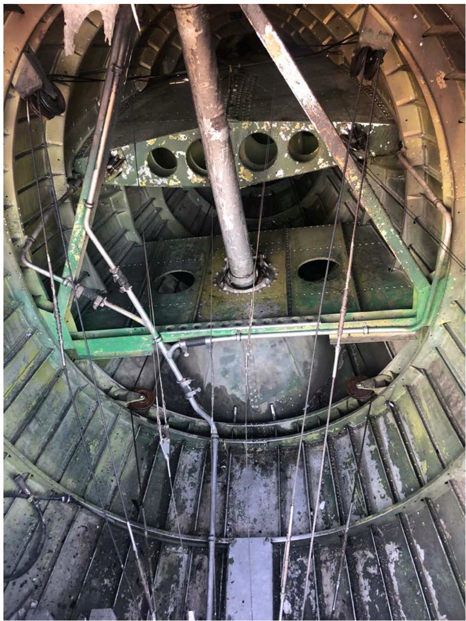
Photo 13 – Aft portion of the fuselage, including the tailwheel insert.
