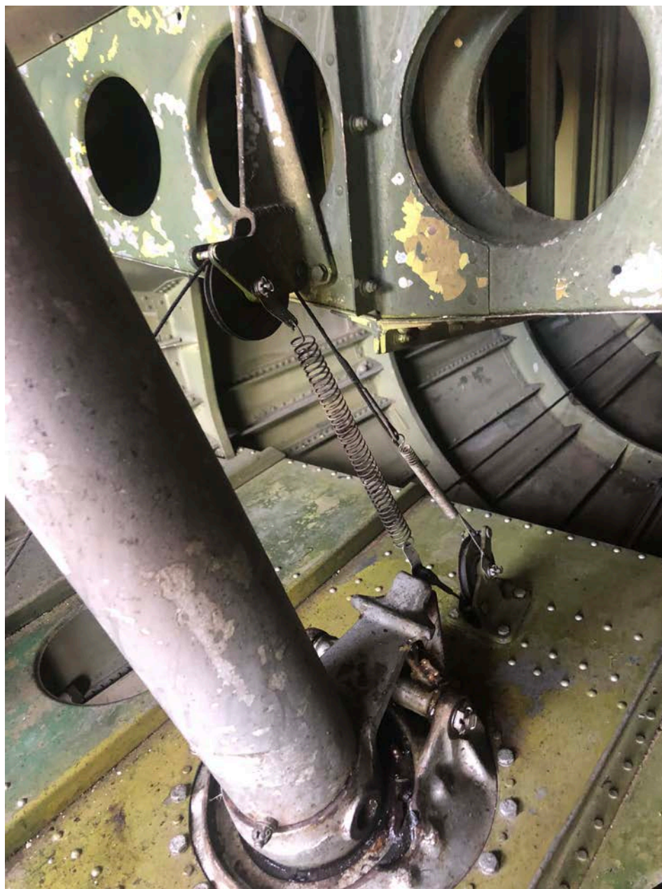
Photo 14 – Tailwheel locking mechanism.
