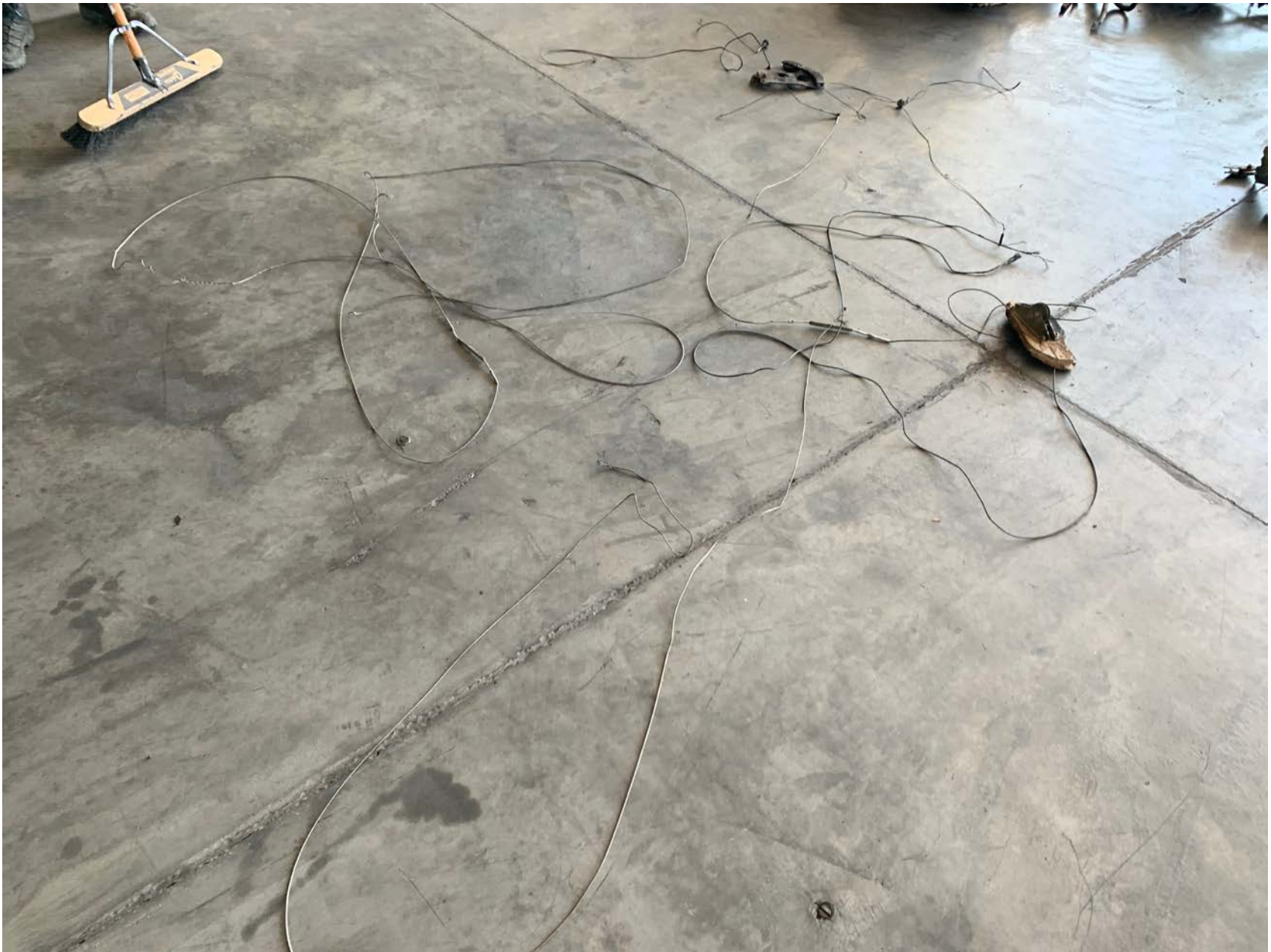
Photo 9 - View of the recovered flight control cables.
