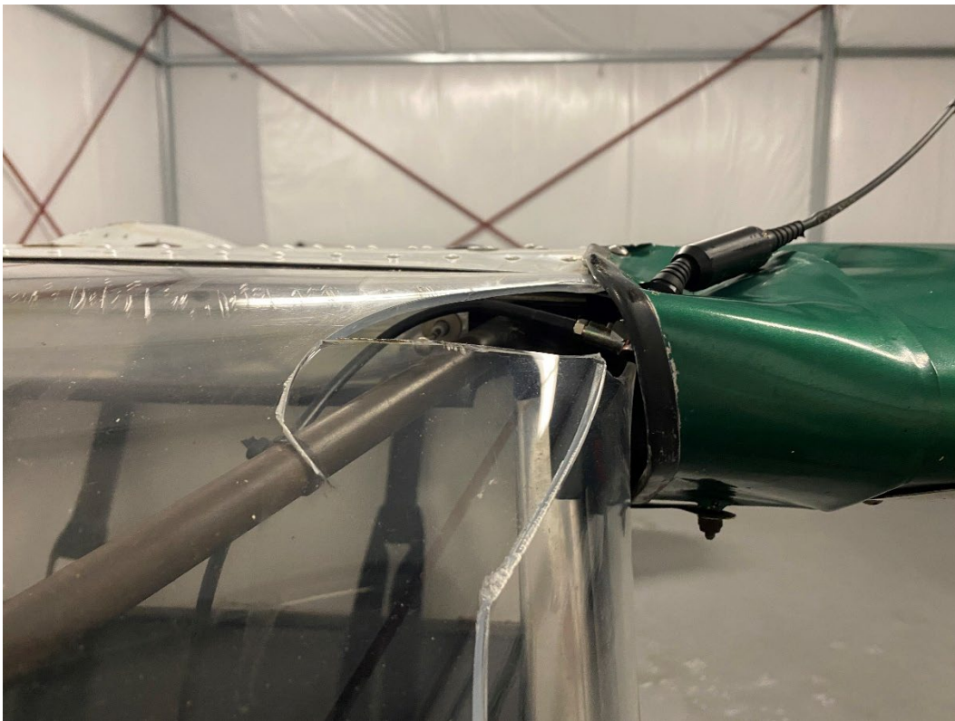
Figure 4: Damage to Wing Root
