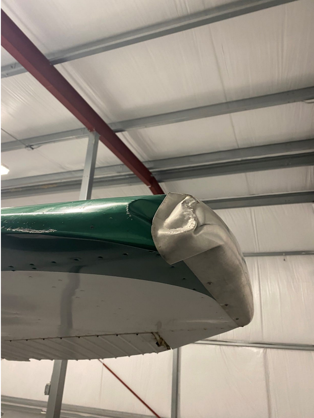
Figure 5: Damage to Left Wingtip
