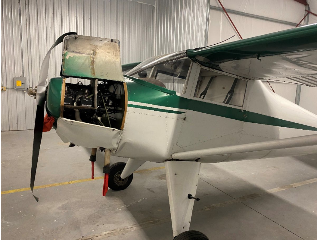
Figure 3: Damage to the Lower Cowling near the Firewall
