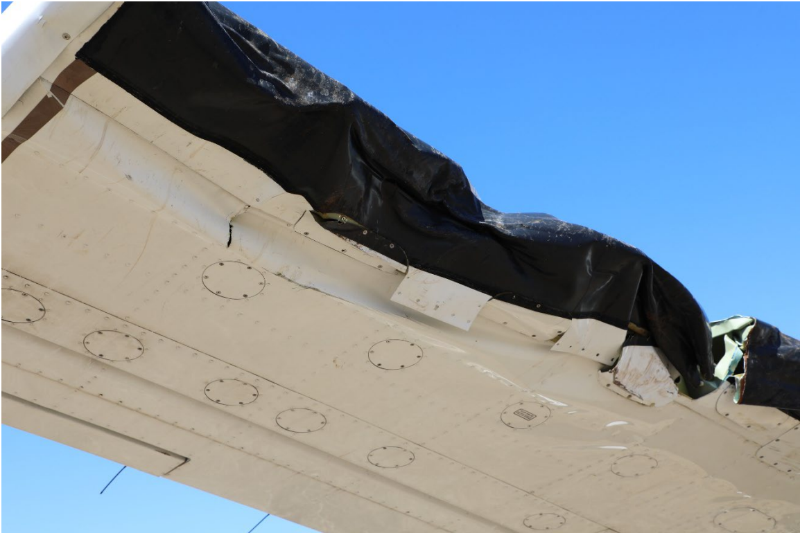
Figure 5: Right-Wing leading edge crush Damage
