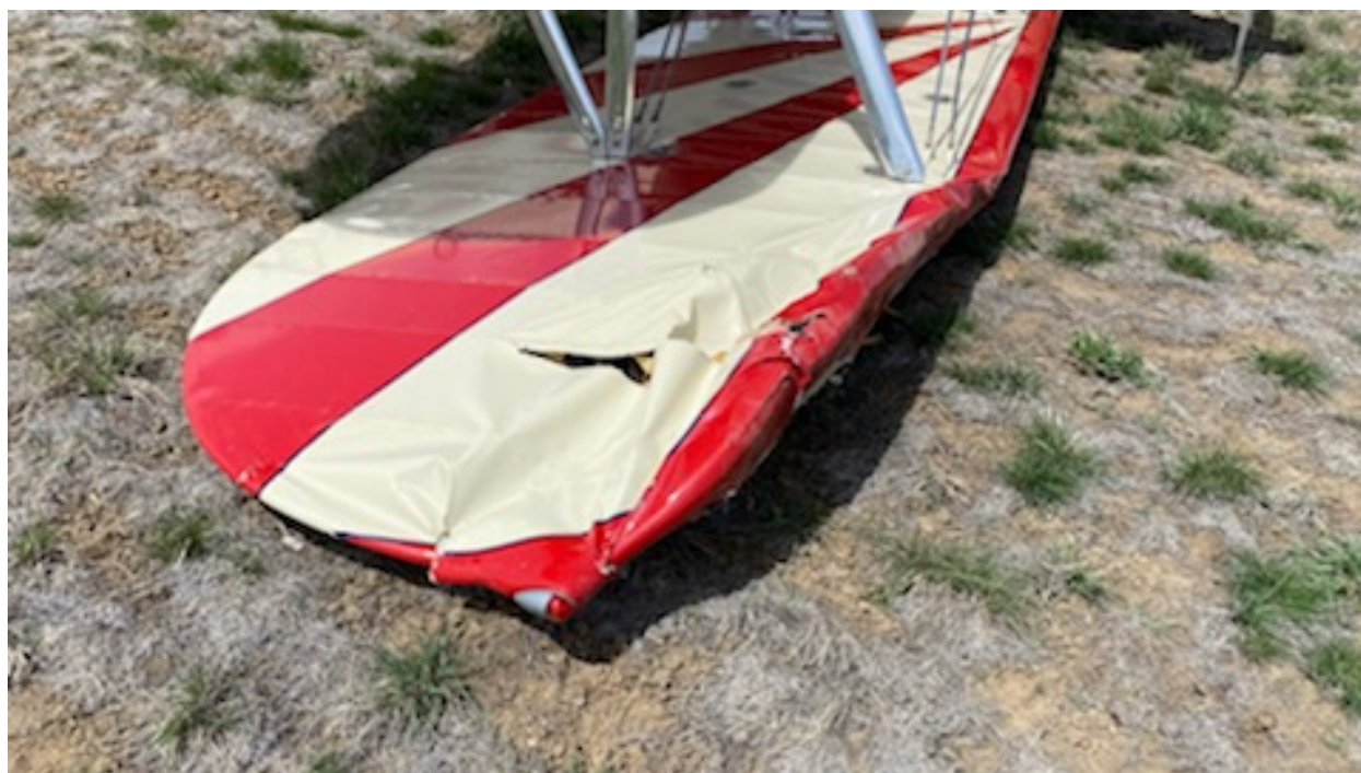
Figure 3: Upper Left Wingtip Damage
