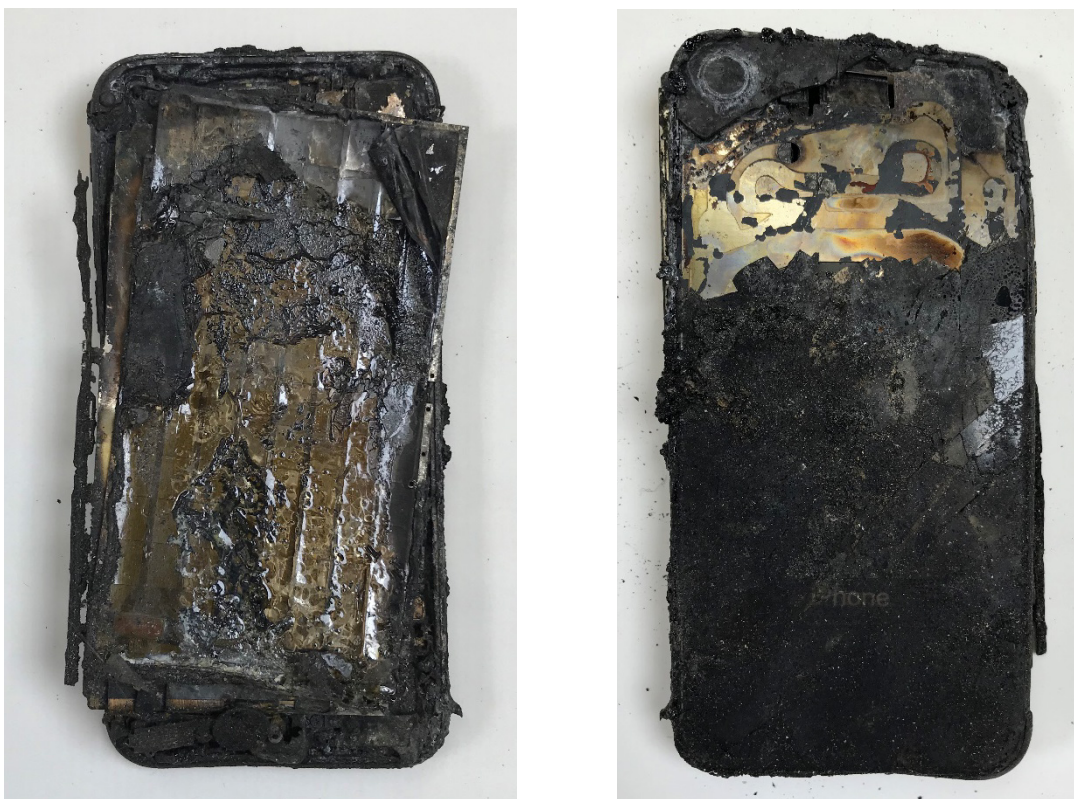
Figure 4. Condition of iPhone 8 as received
