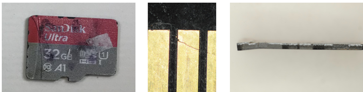
Figure 3. 32GB microSD card recovered after heavy rain from accident site.
