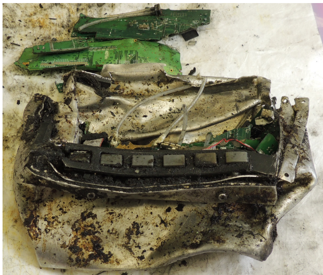
Figure 1. Photo of damaged Dynon device.
