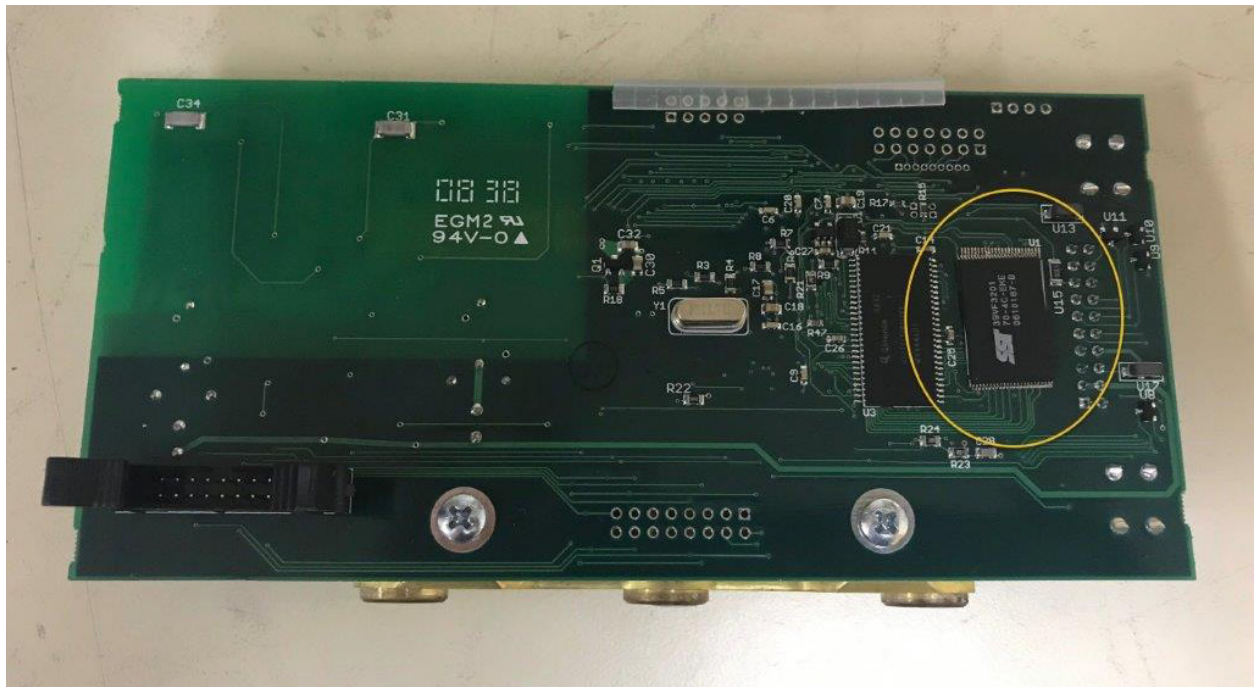
Figure 2. Photo of PCB with NVM installed - undamaged exemplar unit.
