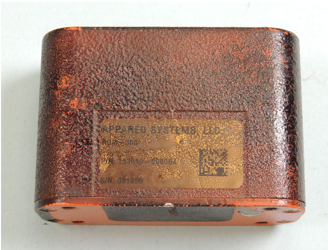
Figure 1. RDM-300 showing heat damage.
