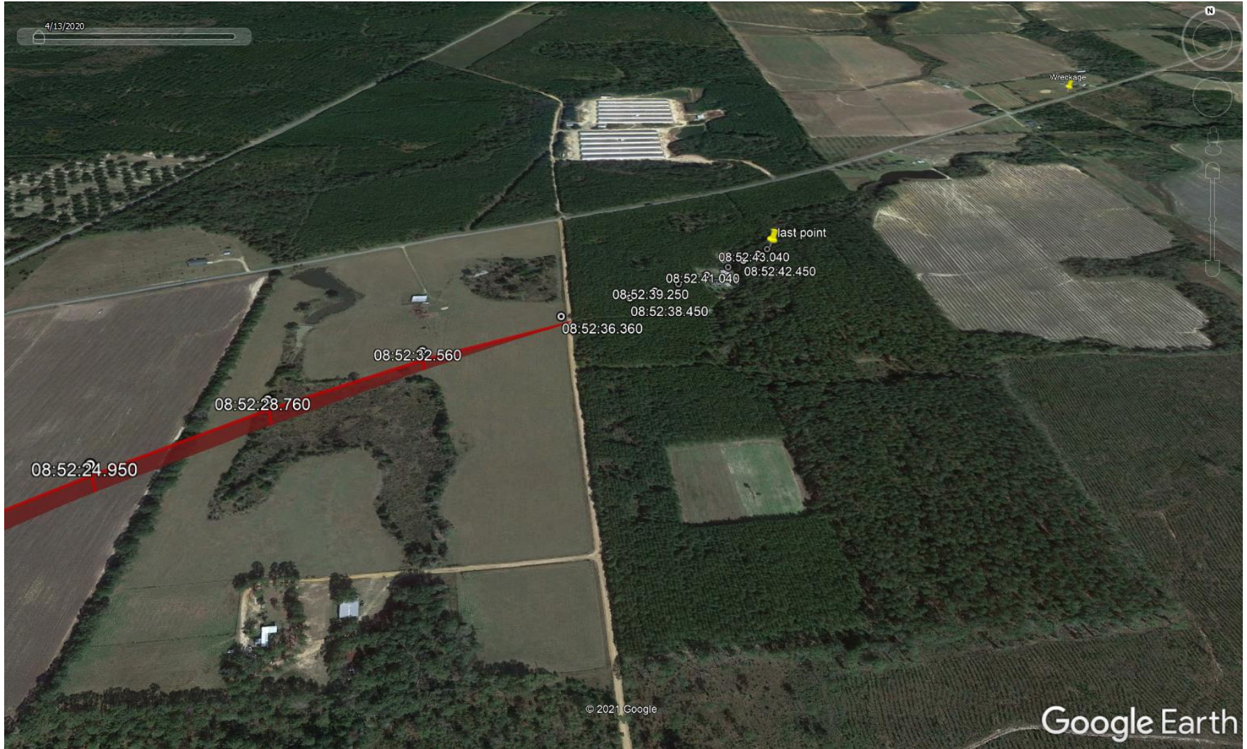
Figure 3. Google Earth overlay showing a north-up overview of the final recorded accident flight track. The last data point is displayed as well as a yellow pin indicating the final resting point of the wreckage.
