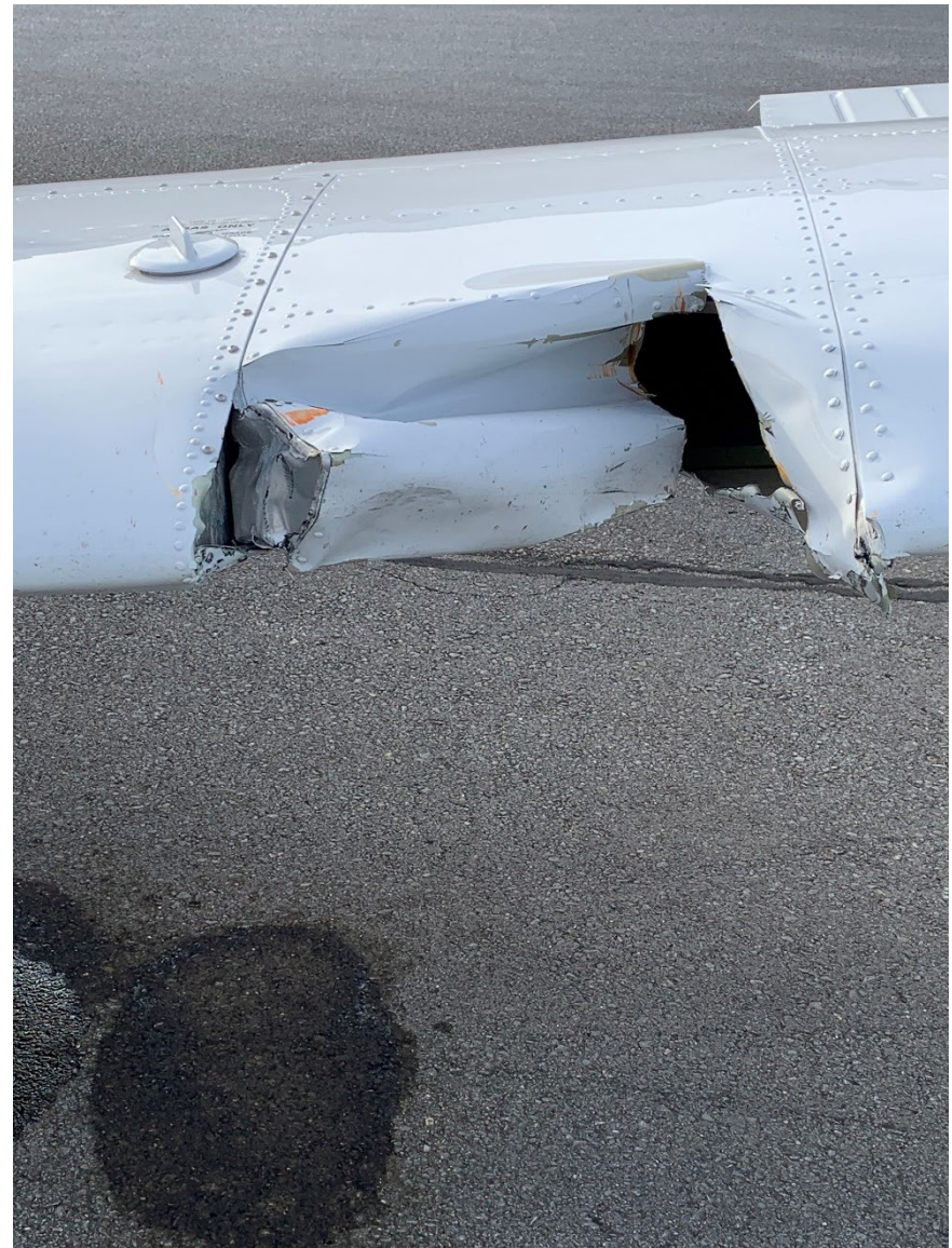
Figure 2: Close View of Left Wing Damage
