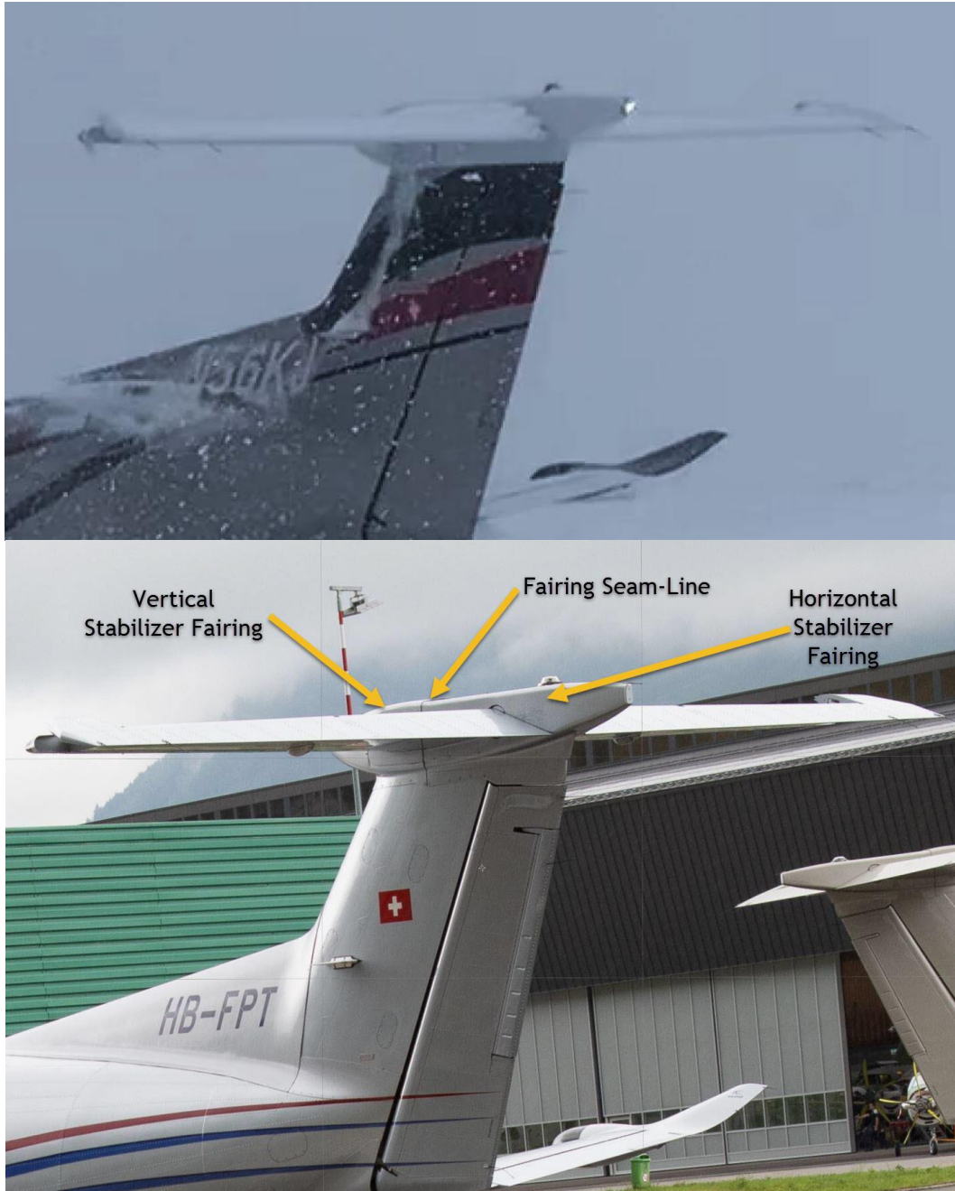
Figure 7. A comparison between a still image from IMG_7378.mov (top) and a photo of an exemplar PC-12 (bottom) taken from a similar angle.
