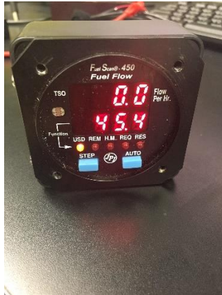
Figure 2. The FS-450 powered to show the amount of fuel remaining.
