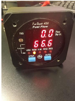
Figure 2. The FS-450 powered to show the amount of fuel remaining.
