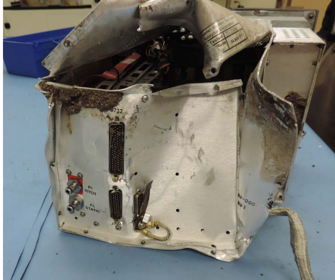
Figure 2. Damaged exterior of PFD – back.
