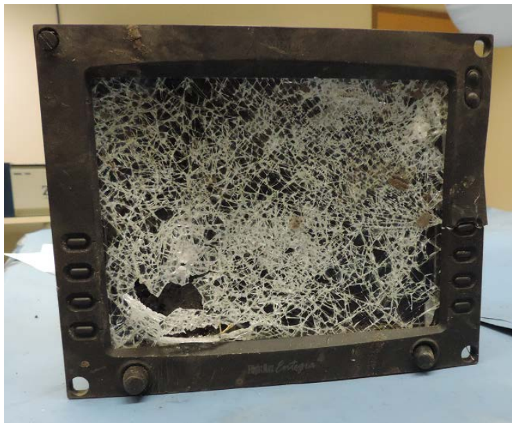
Figure 1. Damaged exterior of PFD - front.
