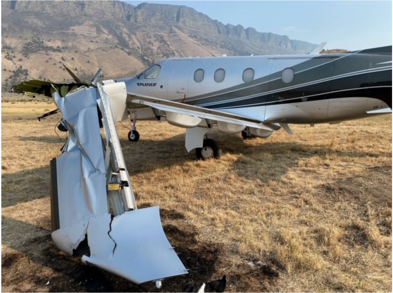
Figure 2: Outboard Left Wing Damage
