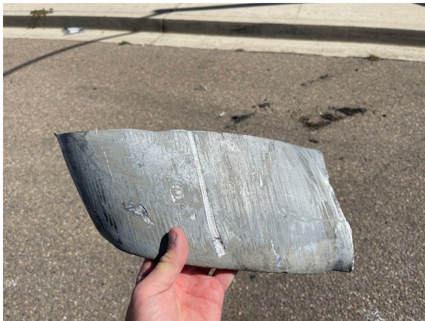
Figure 8: Recovered propeller blade fragment.
