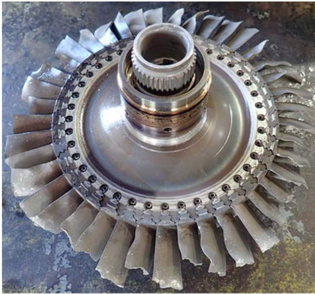
Figure 33. Power turbine downstream face showing heavy rotational scoring and aftward blade displacement
