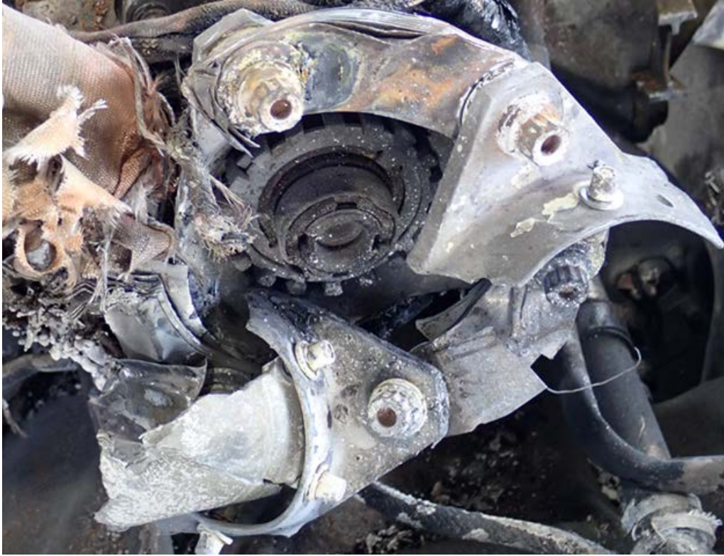
Figure 59. Distorted airframe coupling attached at engine output shaft
