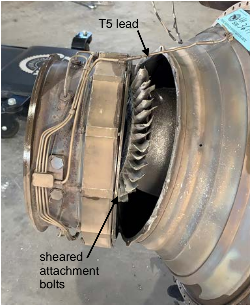
Figure 22. Power turbine stator housing
