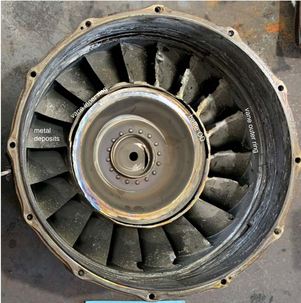
Figure 52. Downstream face of power turbine vane ring and baffle assembly, showing rotational damage
