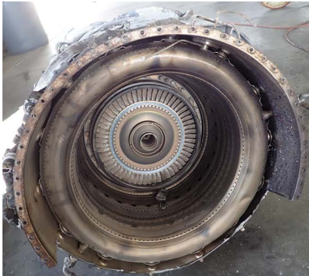
Figure 46. Compressor turbine and combustor after C flange separation
