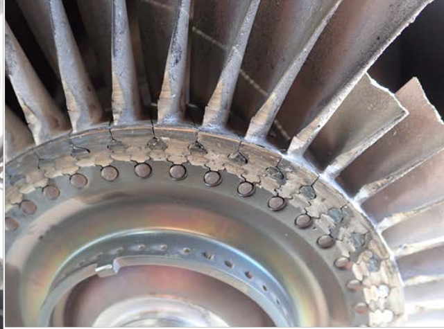
Figure 54. Detail of rotational damage to power turbine upstream face
