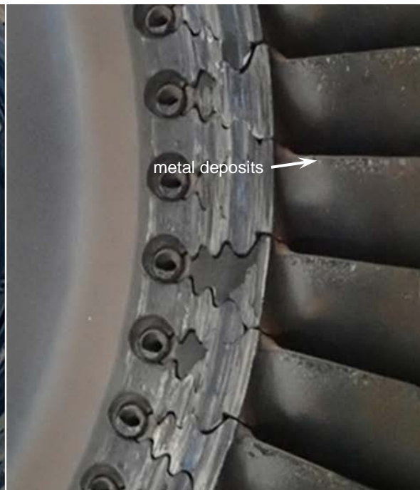
Figure 21. Detail of scoring along blade retention
