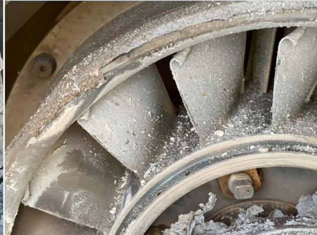
Figure 49. Detail showing curled blade tips
