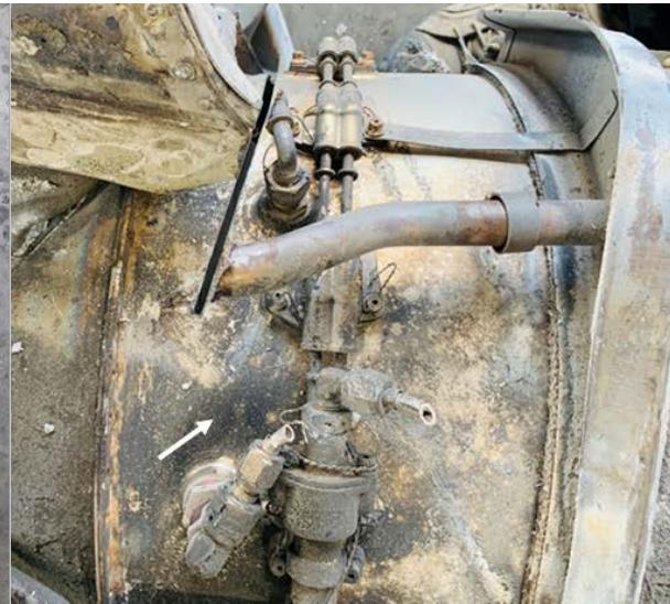
Figure 44. Dented gas generator case
