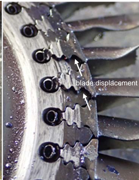
Figure 34. Closeup of power turbine fir tree root area
