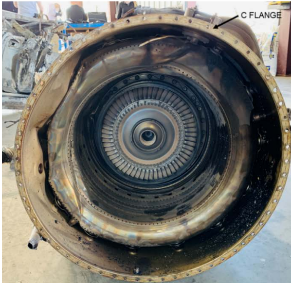
Figure 16. Compressor turbine and combustor exposed by C flange separation
