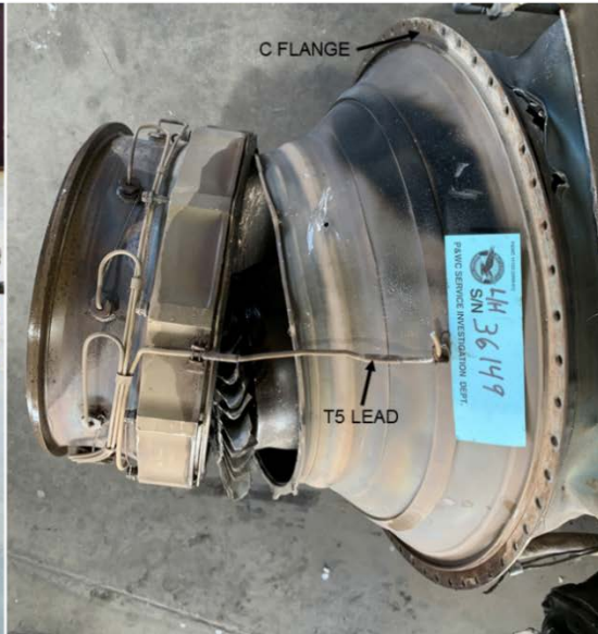
Figure 17. Power turbine stator housing after separation from the gas generator section
