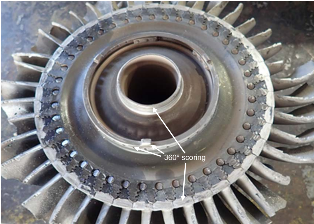
Figure 30. Power turbine upstream face showing circumferential contact damage
