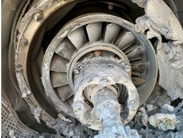
Figure 48. Compressor inlet showing No. 1 bearing package
