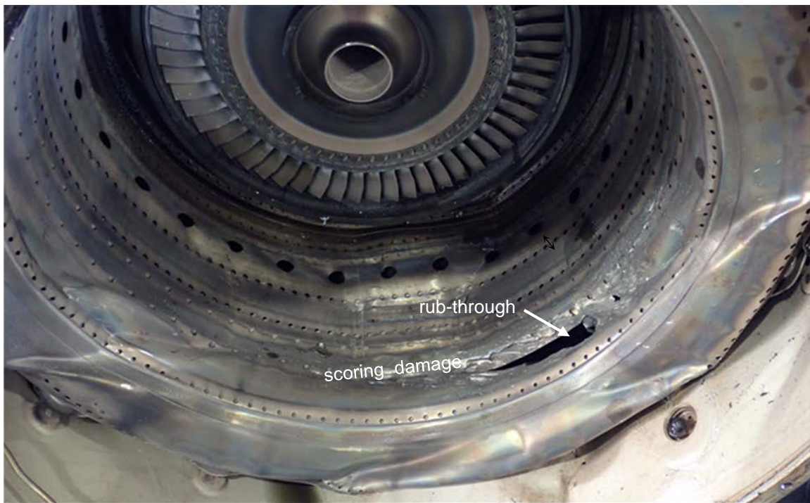
Figure 19. Combustor liner distortion, scoring and metal deposited on shroud segments and blade TEs
