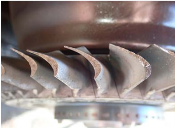
Figure 55. Power turbine blade fracture surfaces
