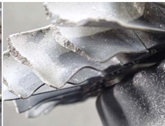
Figure 32. Power turbine airfoil bending
