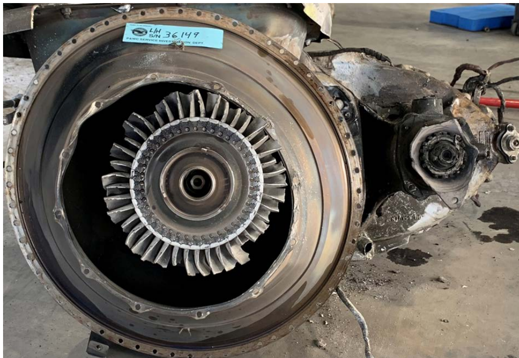
Figure 29. Power turbine with power turbine stator housing removed
