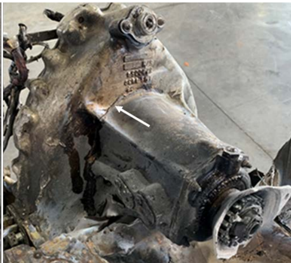
Figure 15. RGB casting fracture
