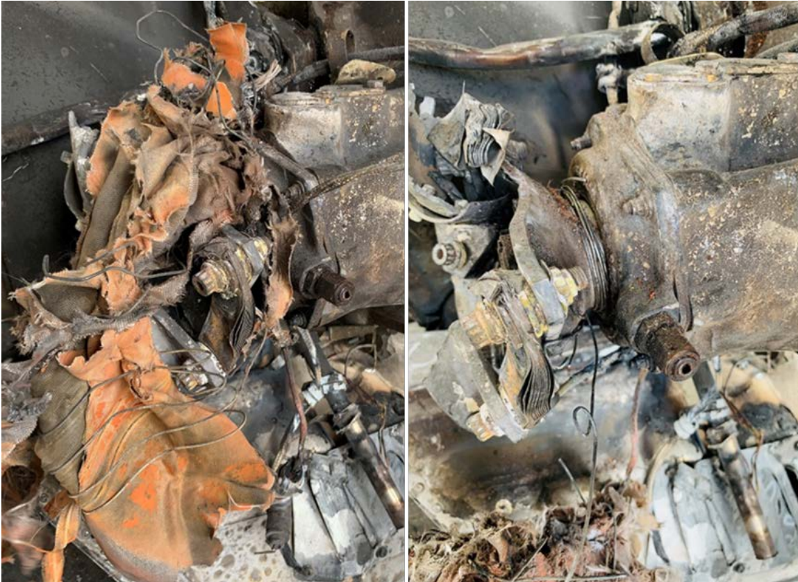
Figure 57. Engine output shaft with hose material Figure 58. Wire wrapped around engine output shaft
