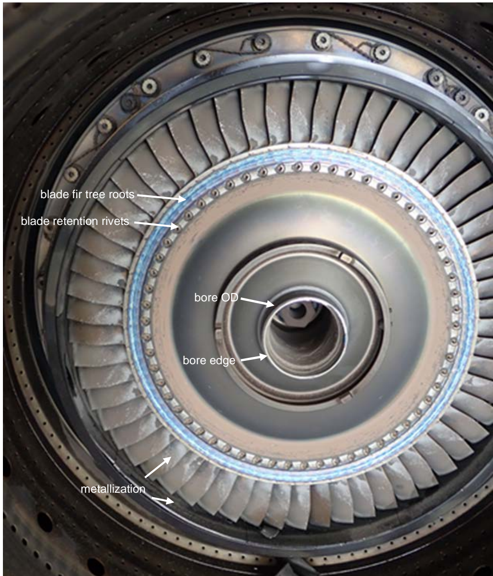
Figure 50. Compressor turbine downstream face showing rub 360° scoring
