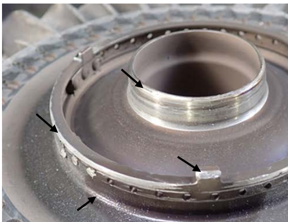
Figure 31. Circumferential damage at bore, bore edge, and tooling lugs
