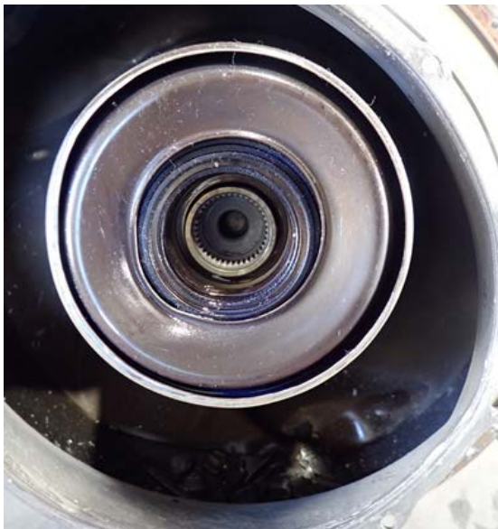
Figure 35. Exhaust duct rotational damage
