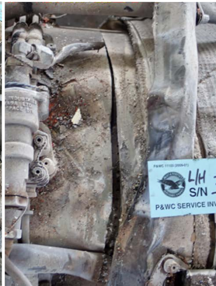
Figure 12. Seam weld fracture in gas generator case
