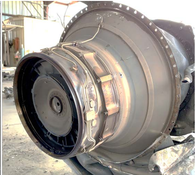
Figure 47. Power turbine stator housing after separation from the gas generator section
