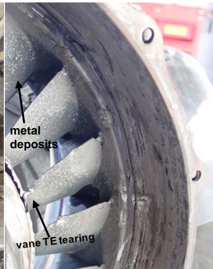
Figure 28. Power turbine shroud
