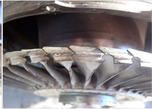
Figure 56. Power turbine blade tip shroud rub damage
