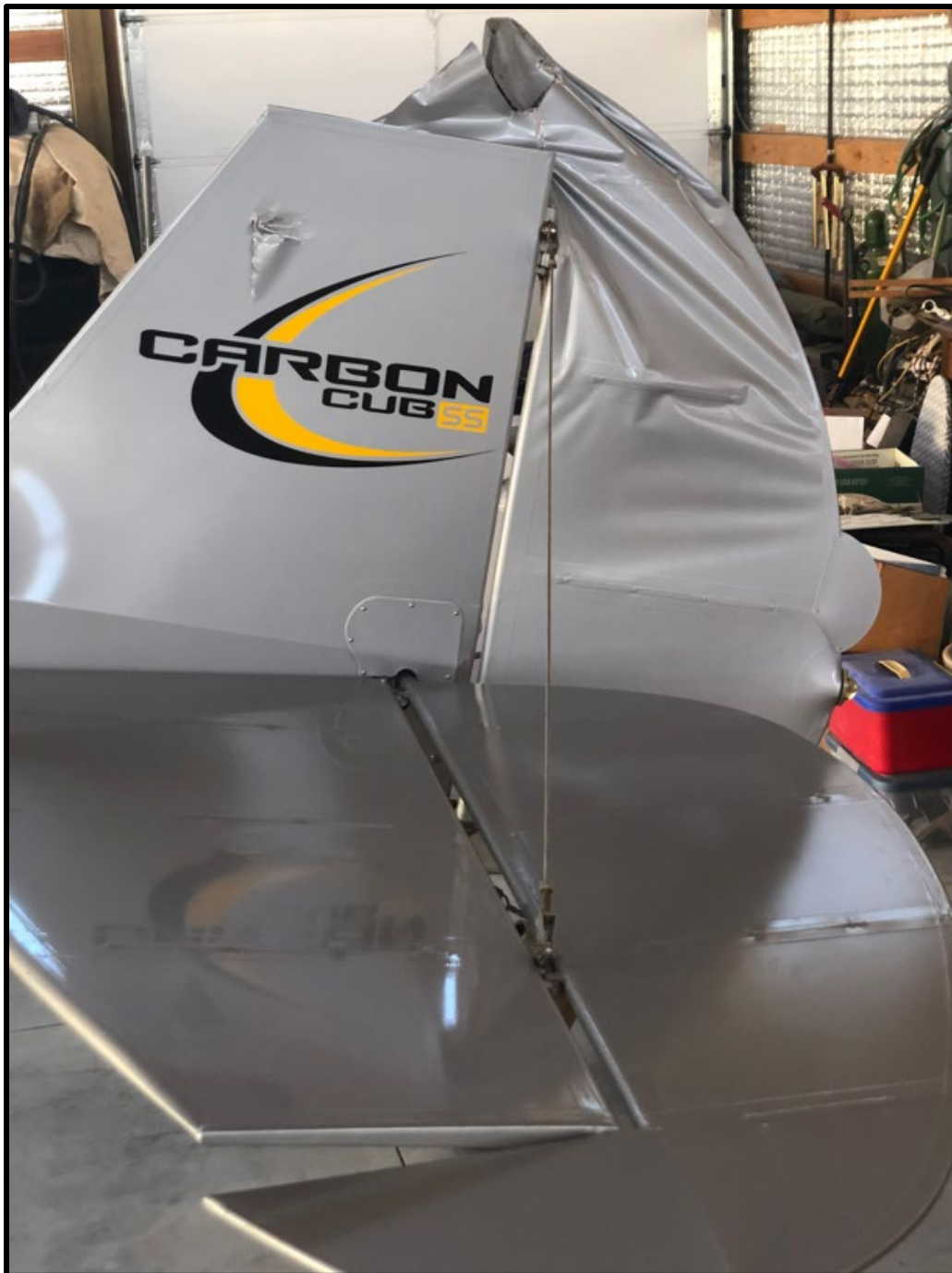
Figure 2: Wrinkled Rudder (photo provided by pilot)
