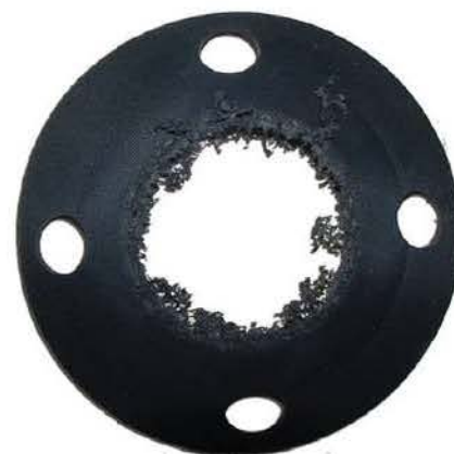
Figure 1. Effects of overcompression on a rubber gasket in a raised-face flange
