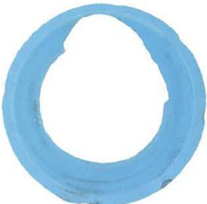
Figure 3. Effects of erosion on a PTFE gasket
