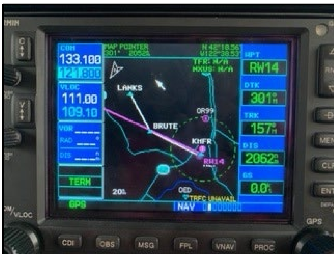
Figure 36: Example of Display on GNS 530W [ignore magenta line and distance]
