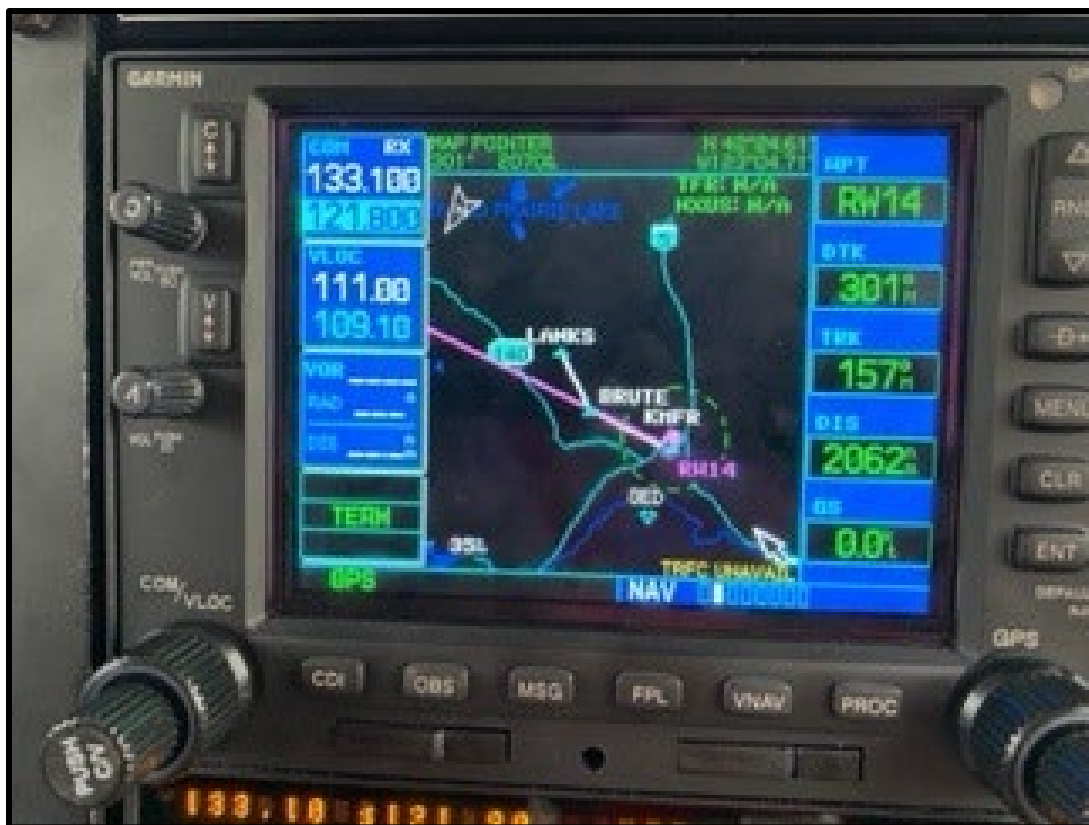
Figure 35: Example of Display on GNS 530W [ignore magenta line and distance]
