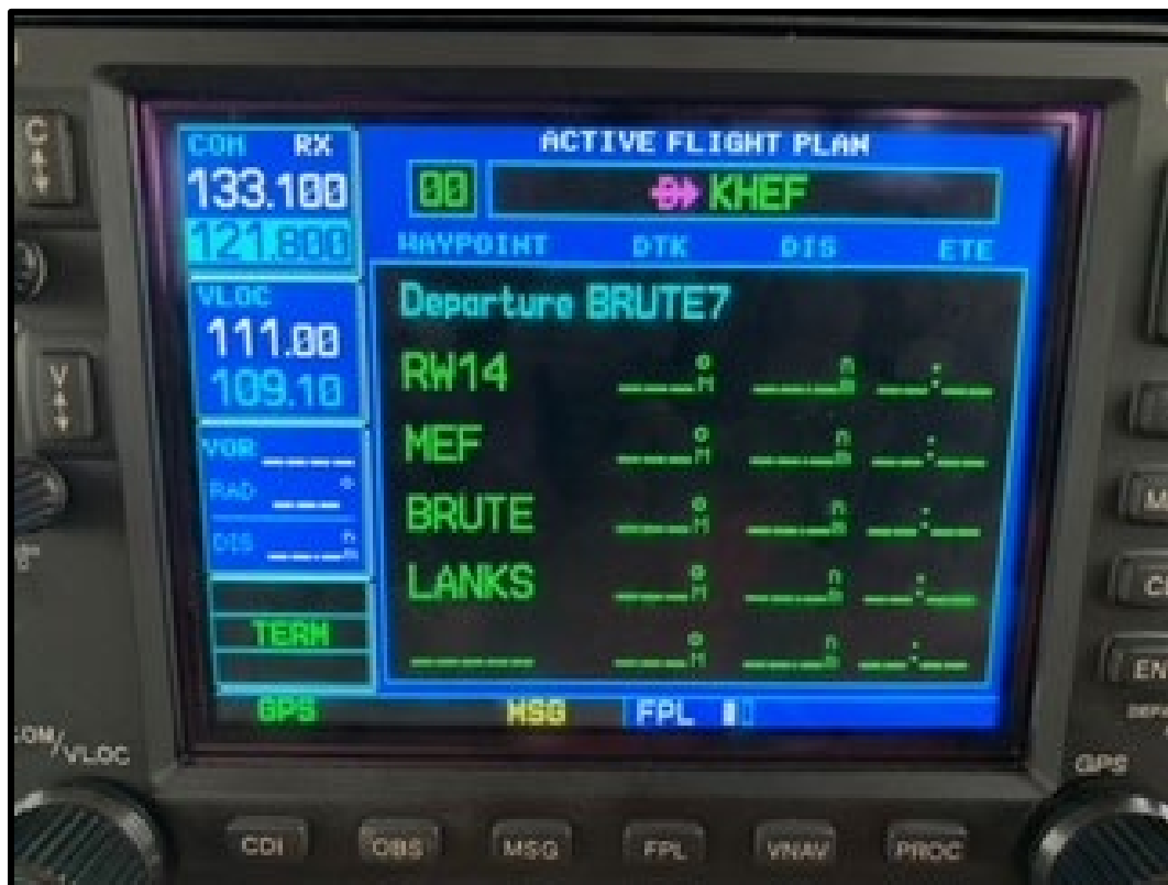
Figure 34: Example of Display on GNS 530W
