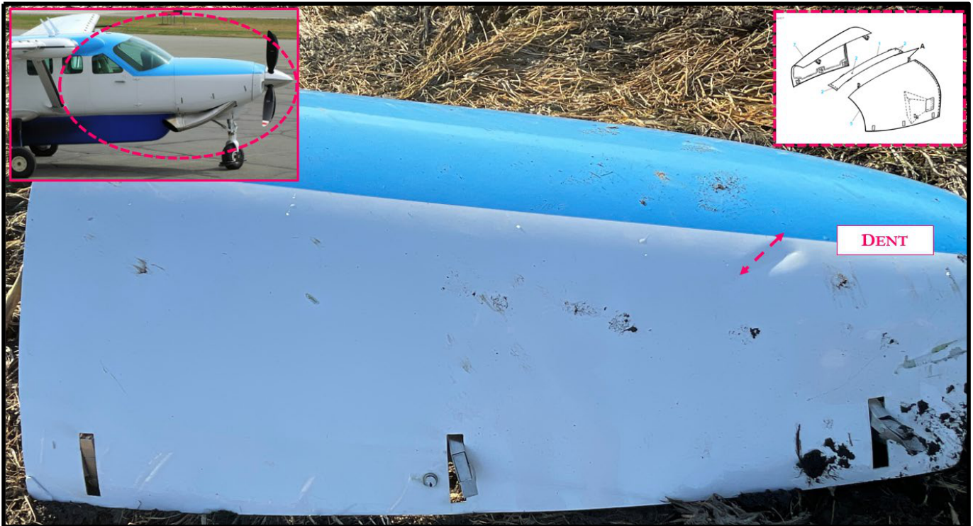
Figure 11: Upper right nose-cowling (photo of the intact airplane provided by Robert Elkelenboom )
