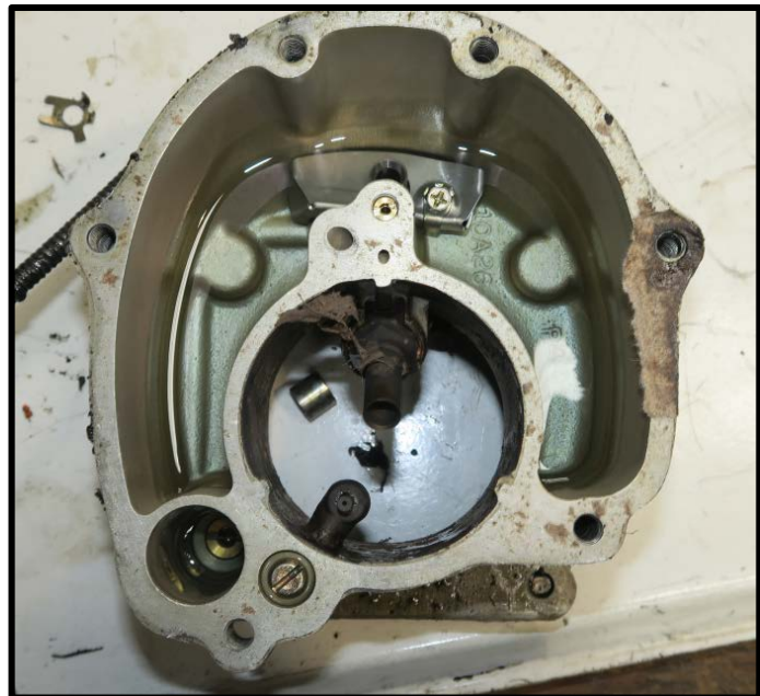
Picture 19: Carburetor Bowl with Fuel
