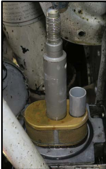
Picture 18: Strainer With Fuel
