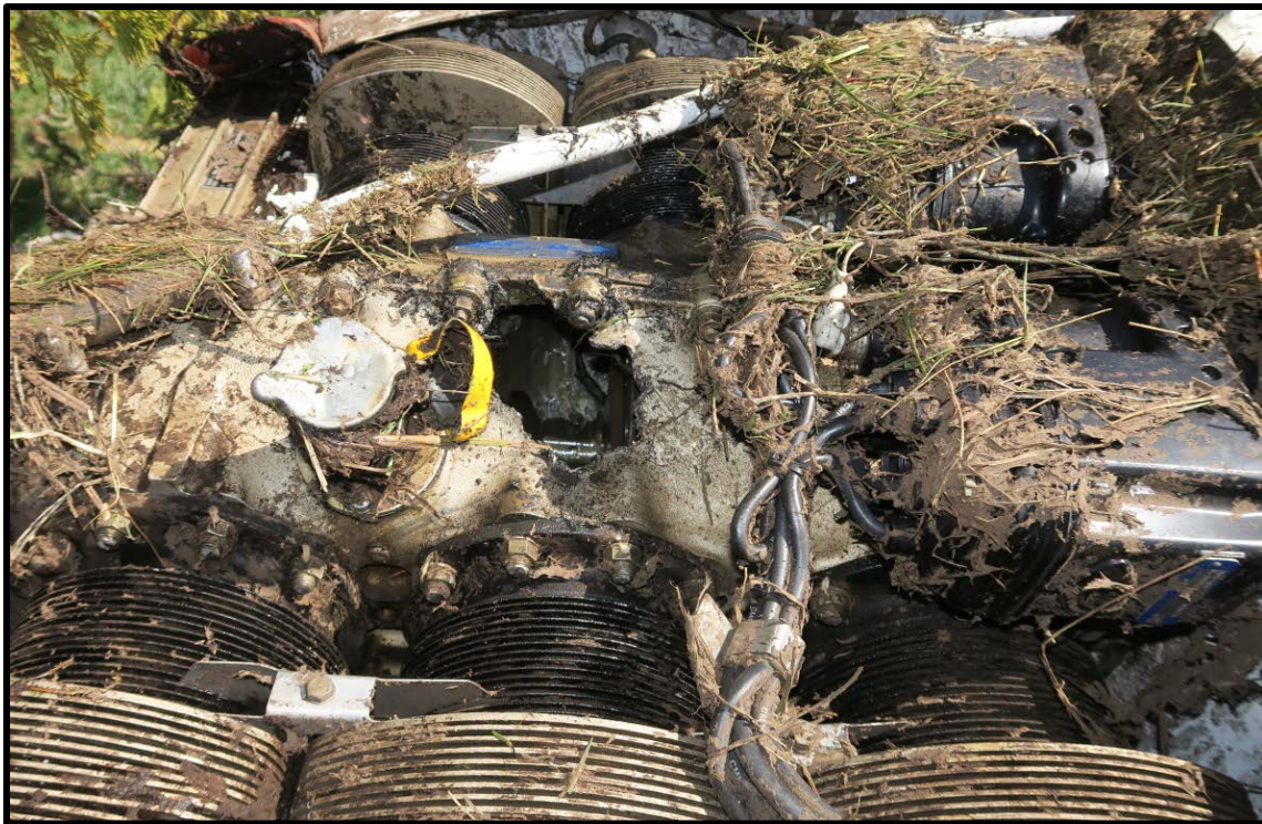
Picture 21: Engine Showing Hole in Case
