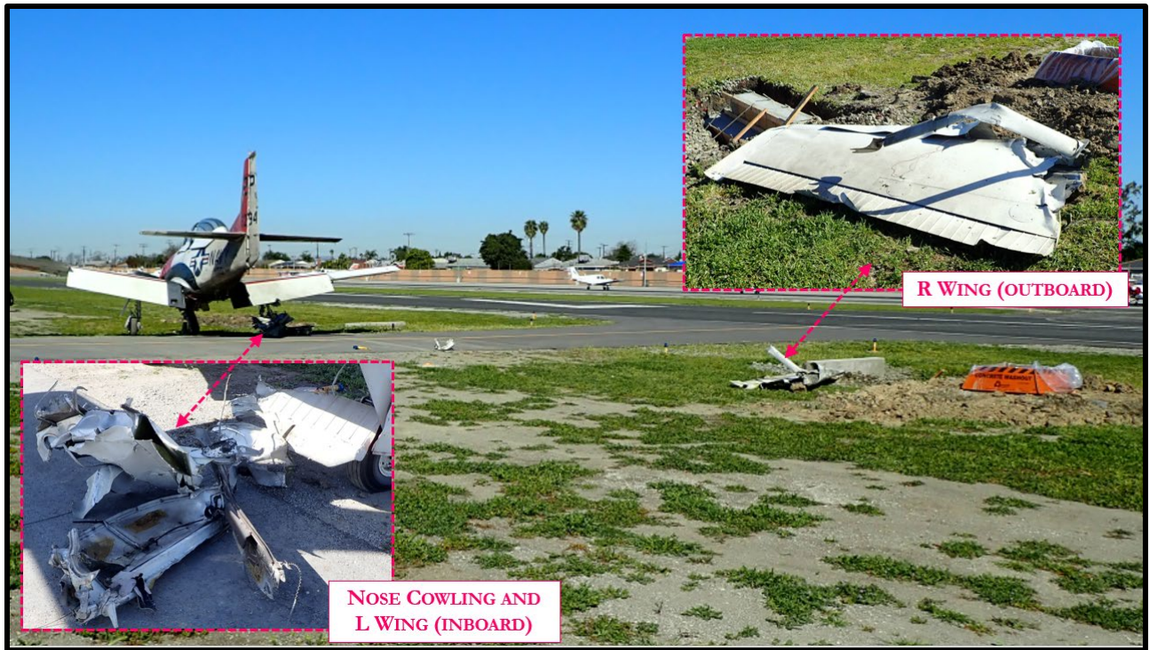
Figure 5: T-28 Debris Field
