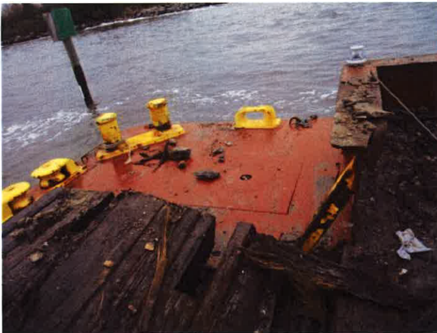
Port stern corner that hit pier
