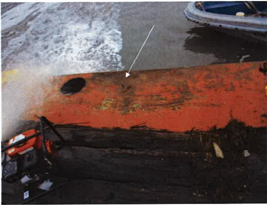
Starboard stern rake deck breech
