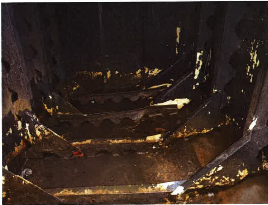
Void 3 upset hull plate, twisted framing
