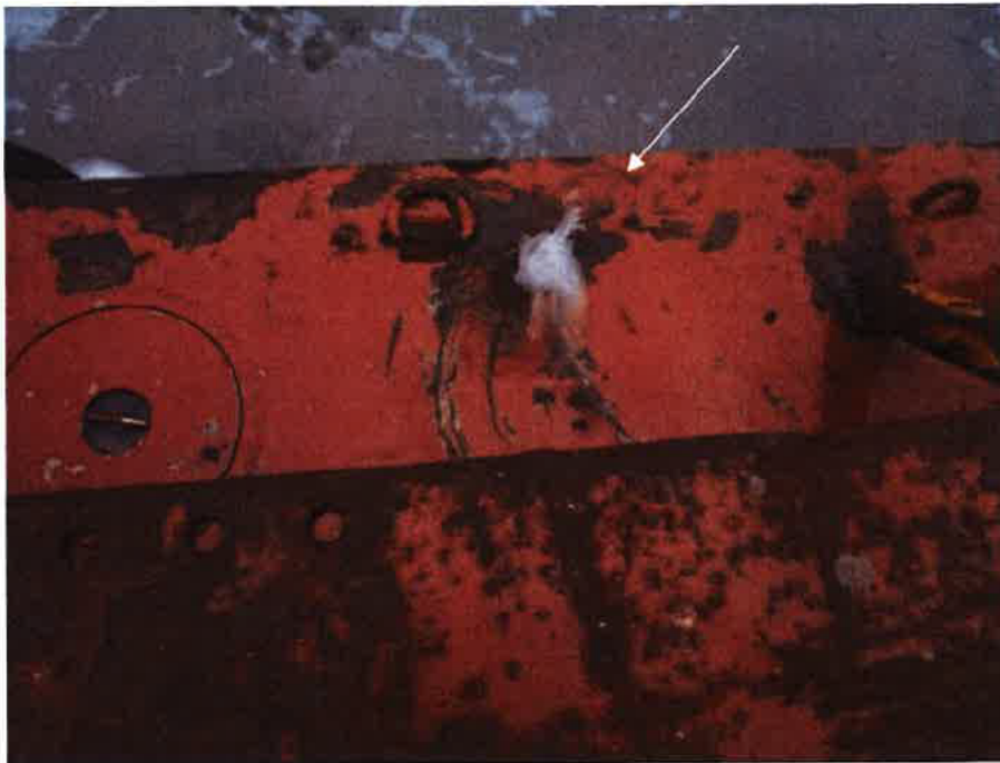
Starboard Void 2 full of water. Water did not drain out when barge was pumped
