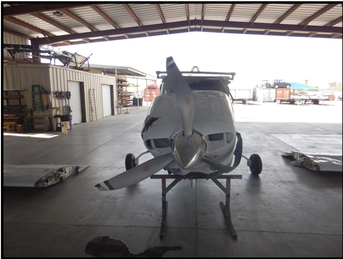
Figure 7: View of the damage to propeller blades (Courtesy of NTSB)
