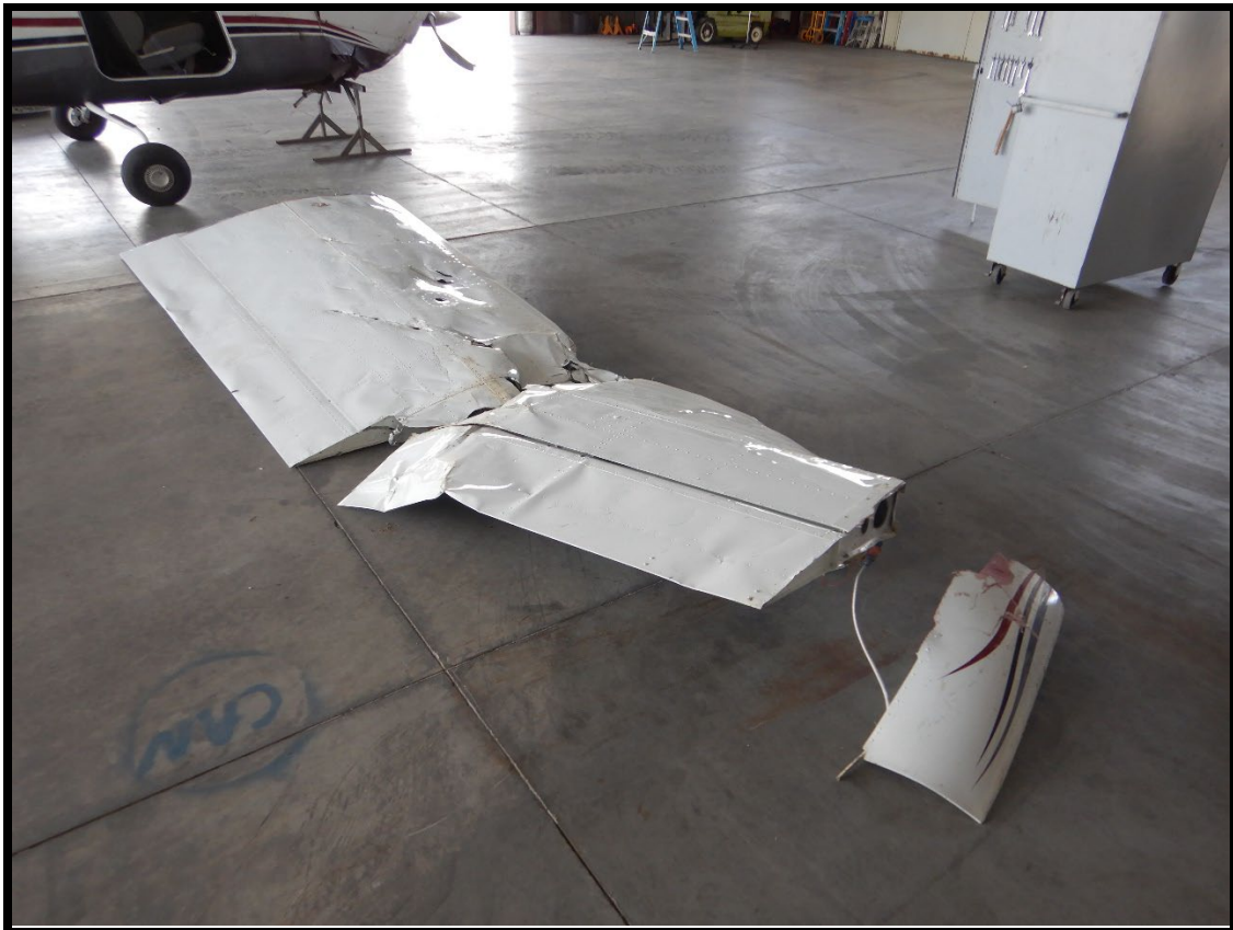
Figure 2: View of damage to right wing (Courtesy of NTSB)
