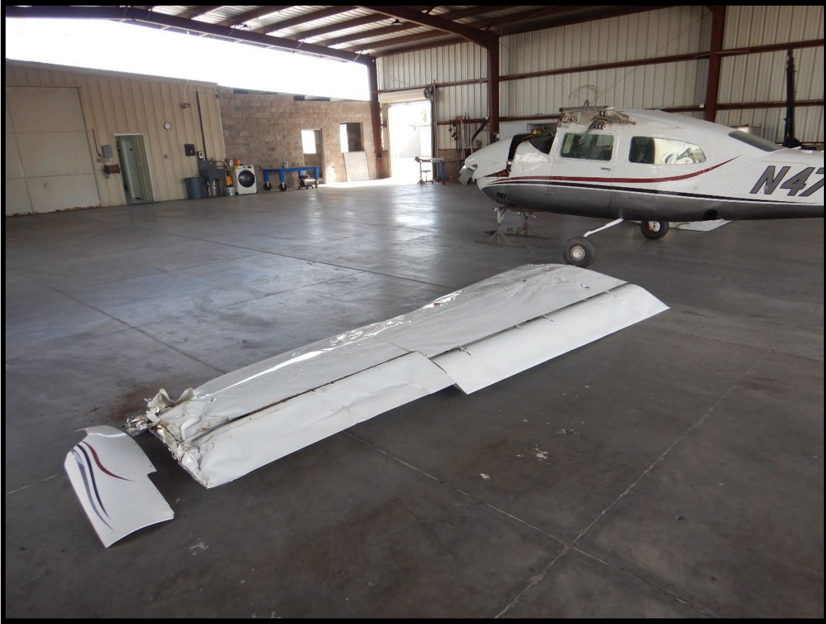
Figure 3: View of damage to left wing (Courtesy of NTSB)
