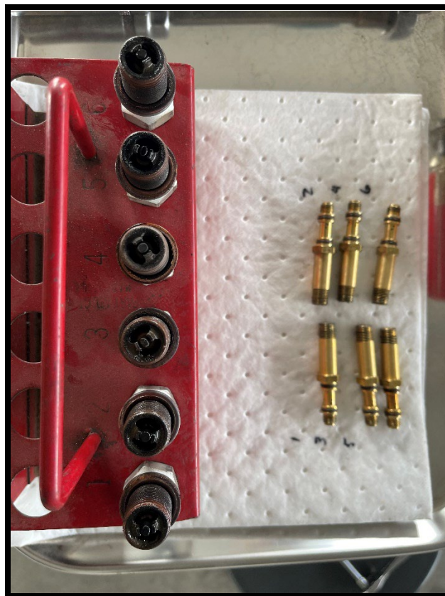
Figure 6: Image of bottom spark plugs and fuel injectors (Courtesy of NTSB)
