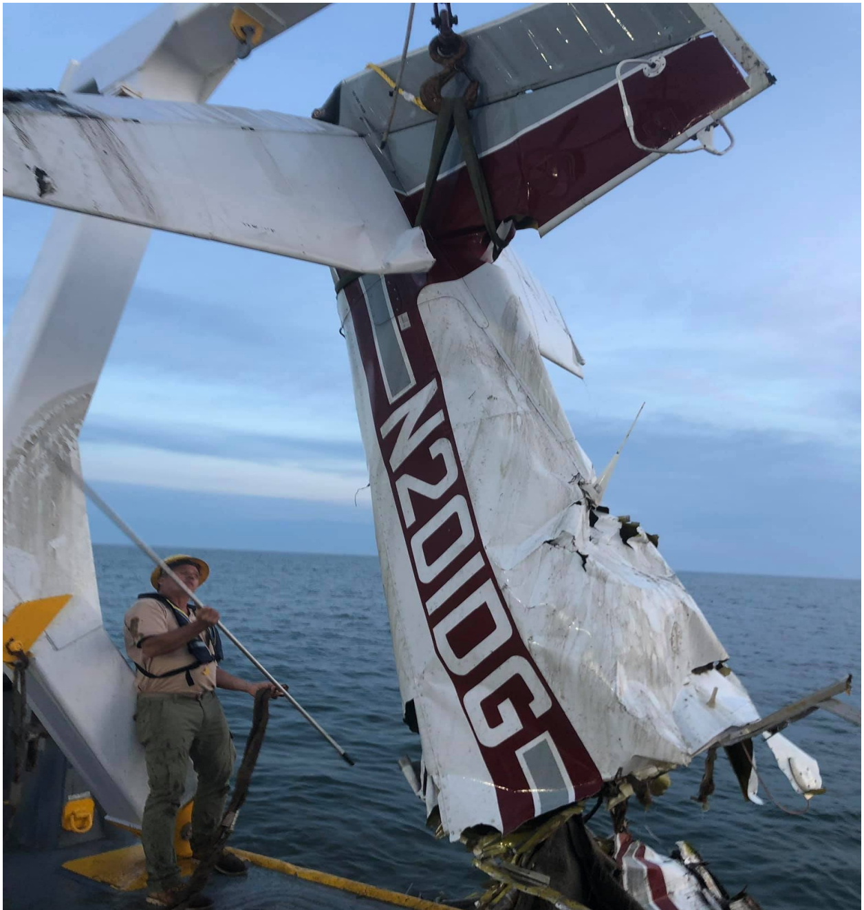
Image 14 – Photograph of the aircraft recovery with the 25 ton A Frame on the Northstar Commander .
