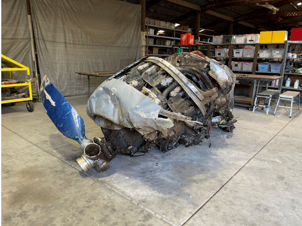
Figure 1: Recovered engine, propeller, and forward portion of the fuselage.
