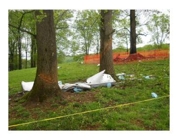
The left aileron and left rudder separated were recovered near the left wing. The right wing and canard remained with the main wreckage and were consumed by fire. The flight controls consisted of control rods and push-pull tubes. Flight control continuity and trim continuity could not be verified due to fire damage.
