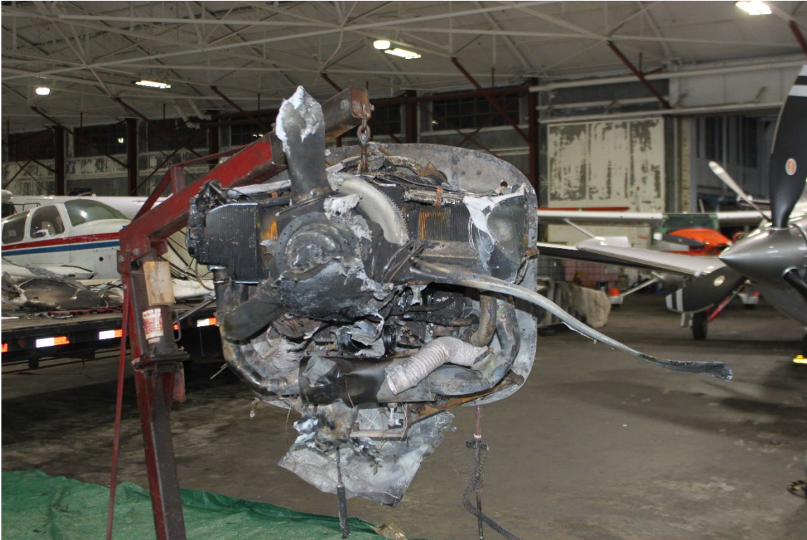
Figure 5: Frontal View of the Engine Assembly with Attached Propeller and Firewall.
