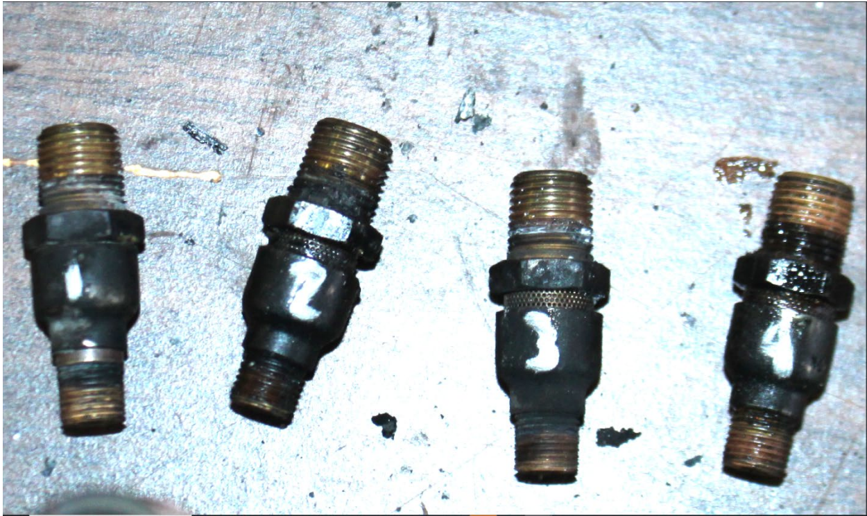
Figure 6: View Following Removal of Fuel Injector Nozzles.
