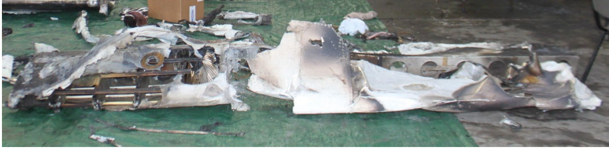
Figure 4: Cropped Image of Remains of Left Wing in Foreground.
