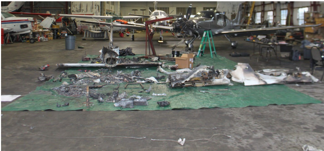
Figure 2: Image of Reconstructed Wreckage.
