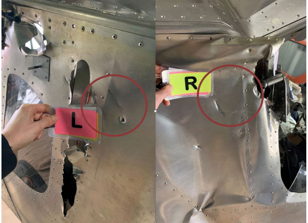
Figure 3. View of contact marks from the inboard flaperon. The orange circle notes the impact mark.
