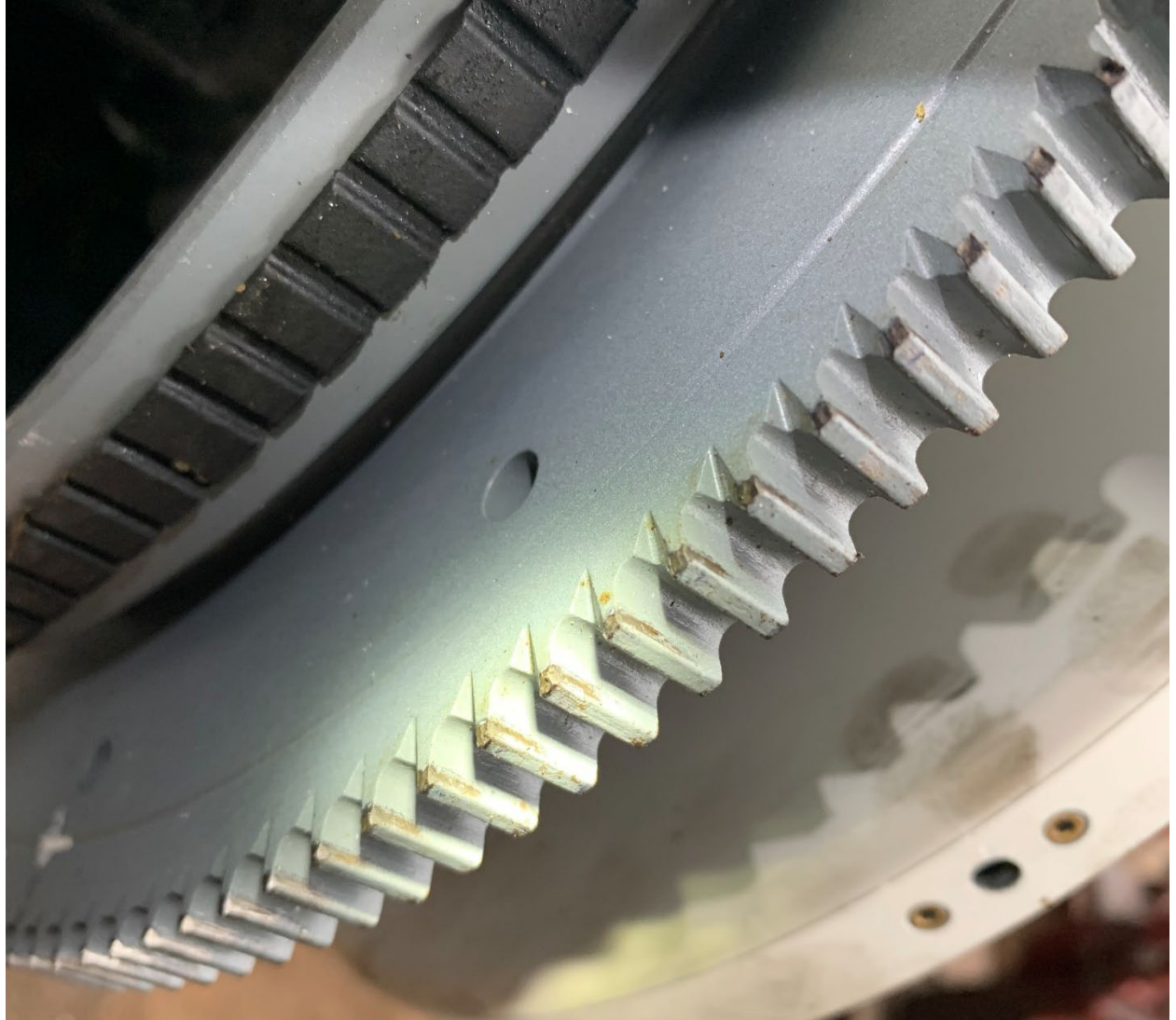
Figure 23. Starter ring gear teeth damage.
