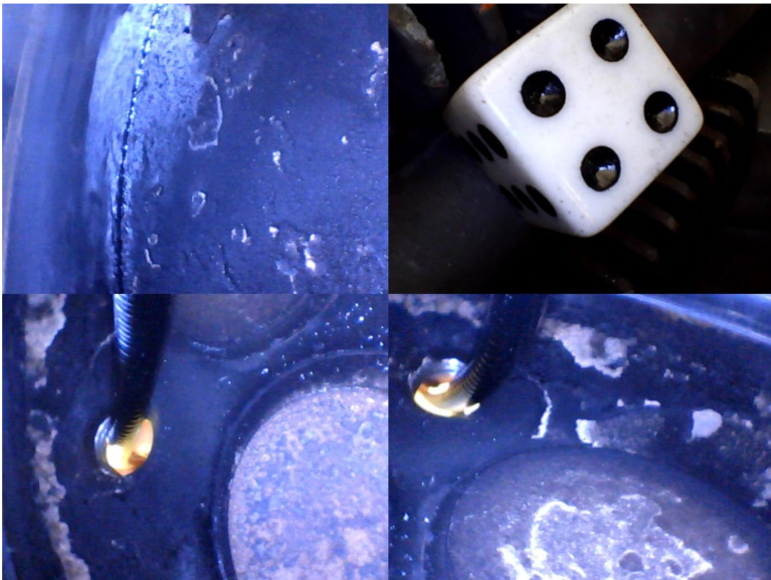
Figure 21. View of piston face and valves of Cylinder No. 4.
