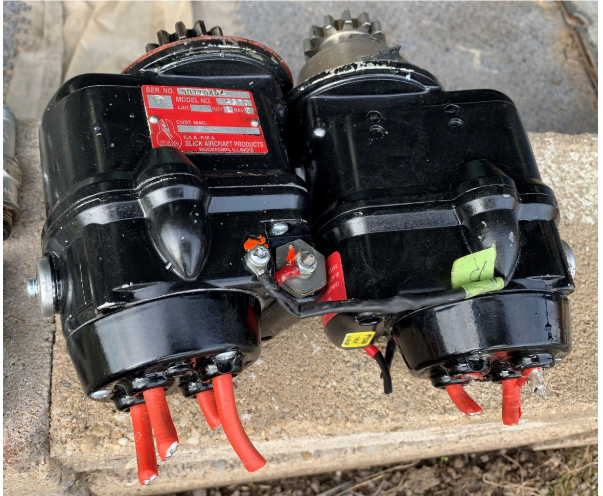
Figure 15. View of both magnetos removed from engine.
