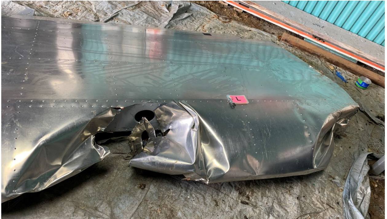
Figure 8. View of left wing semicircular impact damage and wing tip damage.
