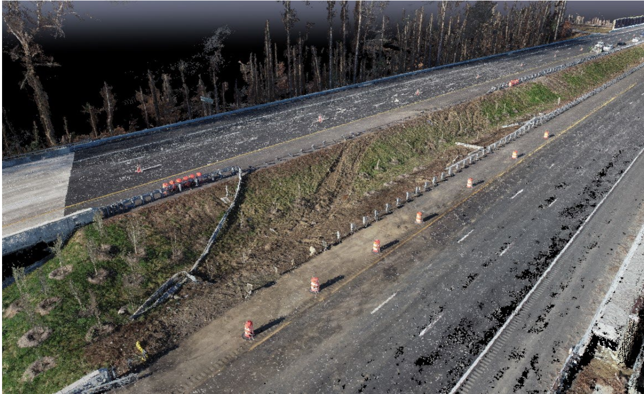
Figure 2. Screen capture of the generated three-dimensional point cloud from Pix4D
