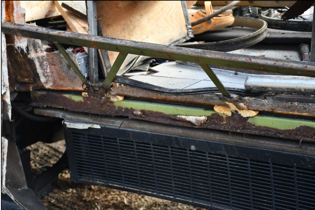
Figure 7: Bus - Corroded Components
