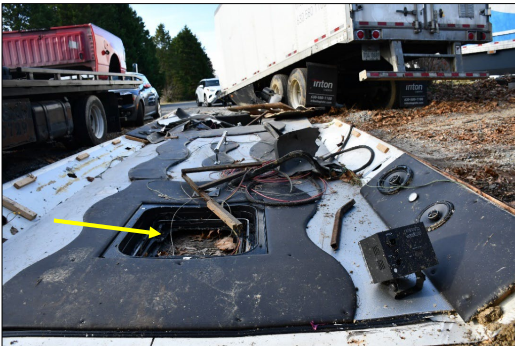
Figure 8: Bus - Roof with Emergency Exit Hatch
