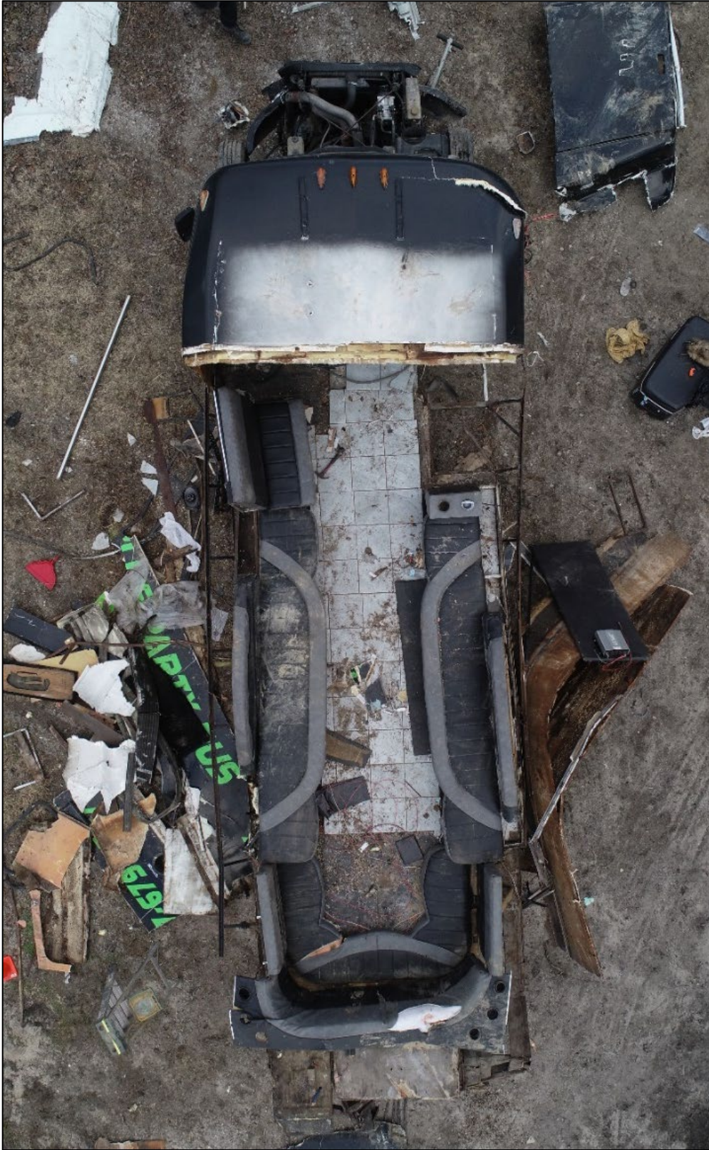
Figure 18: Bus - Aerial View of Reconstructed Seating Arrangement
