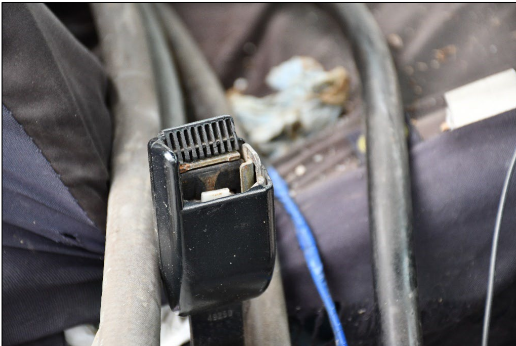
Figure 12: Bus - Damaged Seatbelt Buckle
