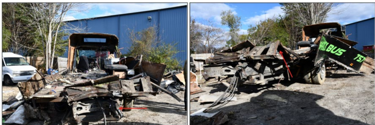
Figure 4: Bus - Damaged Right C-Channel & Buckled Floorboard
