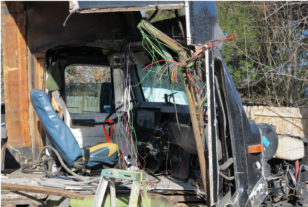
Figure 4: This is where the wiring for the rear of the bus was either severed or cut.
