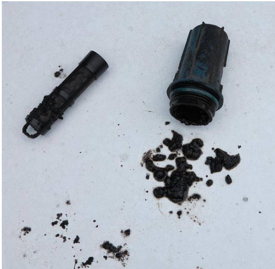
Figure 2: Pre-Screen Element and Debris
