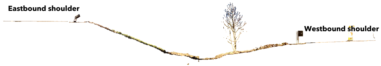
Figure 2: Cross-sectional image of median within the area traversed by the Freightliner combination as rendered in the 3D point cloud.
