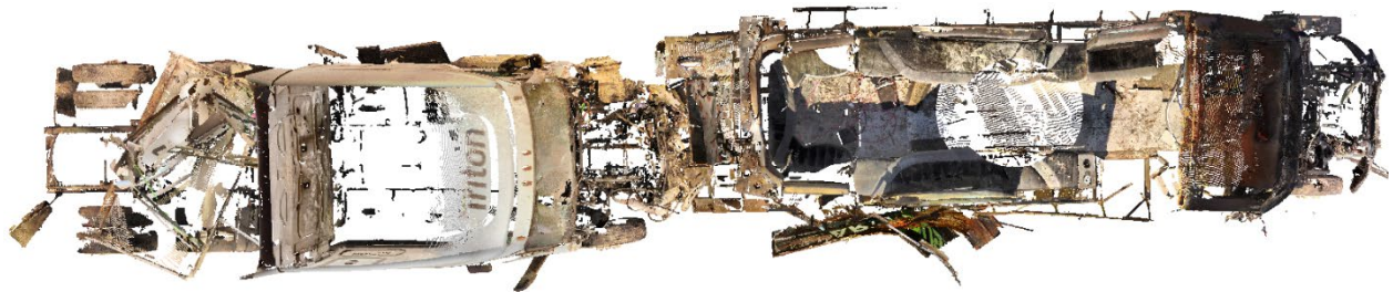
Figure 11: Screen capture of the alignment of areas of contact for the Freightliner and Eldorado bus.
