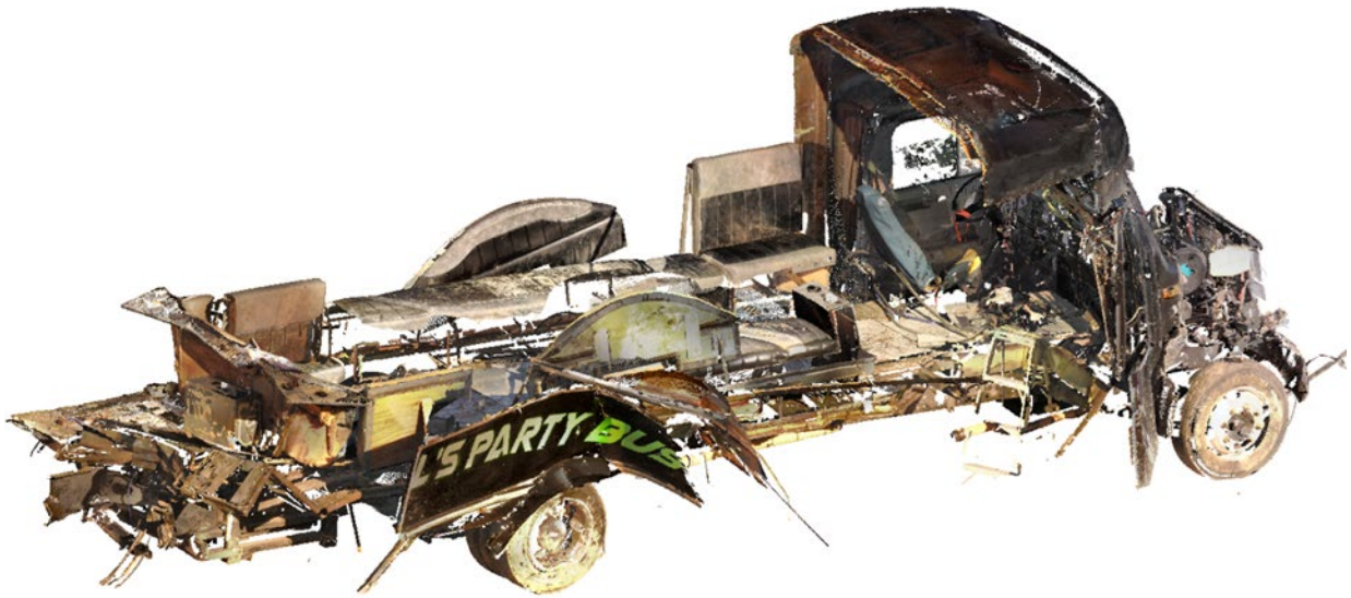
Figure 10: Screen capture depicting an oblique view of the Eldorado bus 3D point cloud
