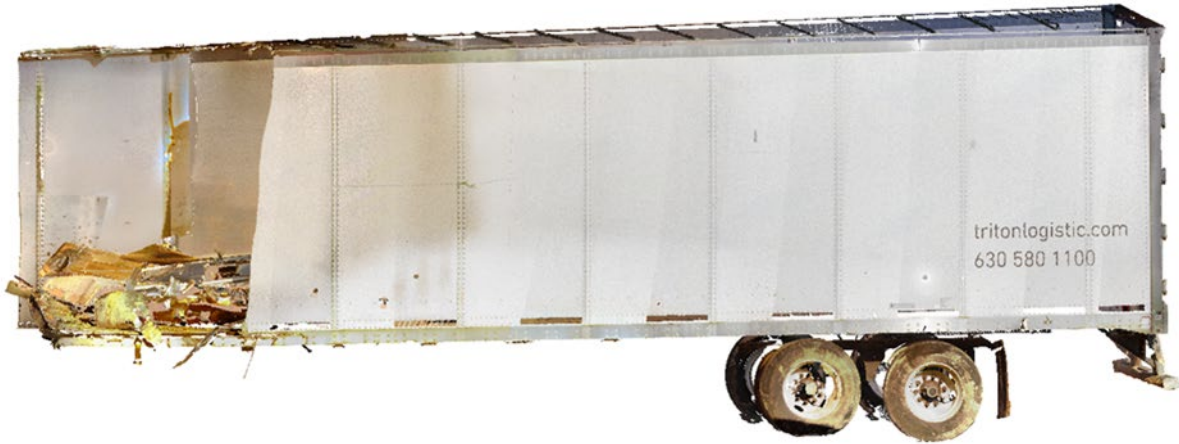
Figure 9: Screen capture depicting a left side view of the Great Dane semitrailer 3D point cloud.
