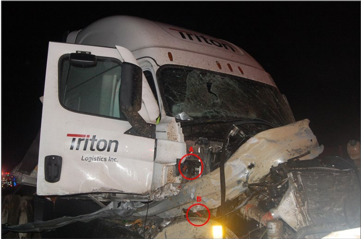
Figure 12: Photograph provided by VSP investigators depicting the Freightliner truck tractor at its position of rest at the crash scene depicting the W-beam guard rail uprooted from the eastbound roadway draped across the engine compartment. Circle "A" indicates the position of the Battery Cable Access (BCA) box while circle "B" highlights a portion of the battery cable that ascends the firewall to the BCA.
