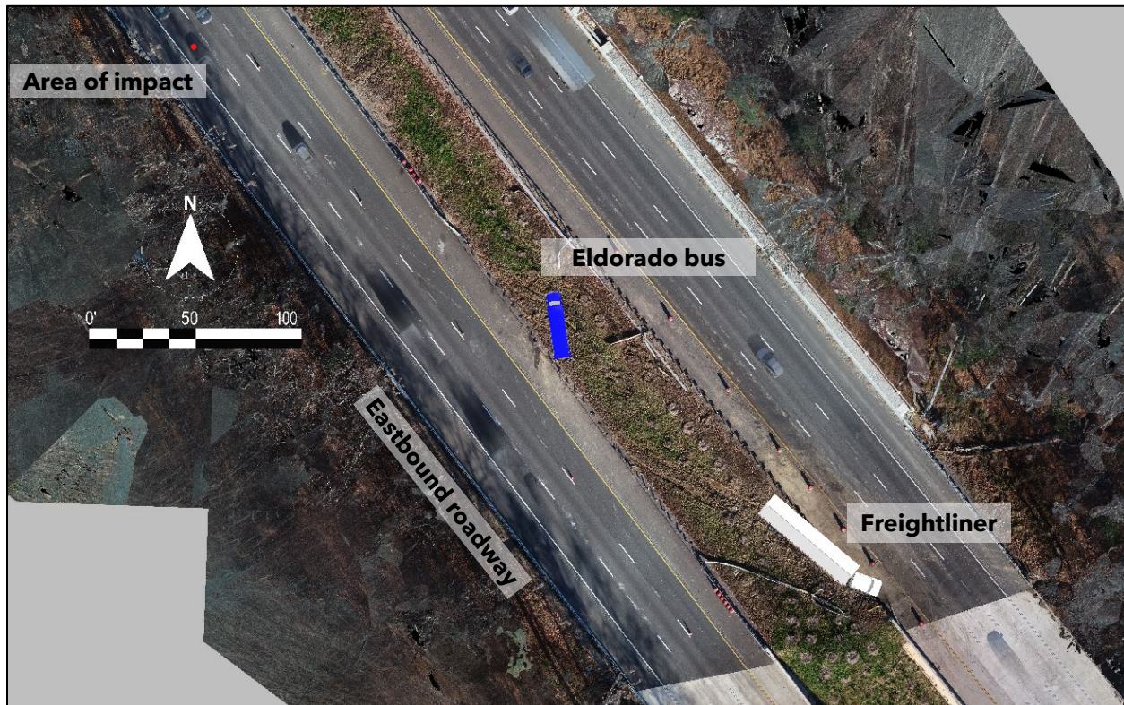
Figure 6: Screen capture depicting a cropped portion of the photogrammetry project orthomosaic image highlighting the vehicle positions of rest.
