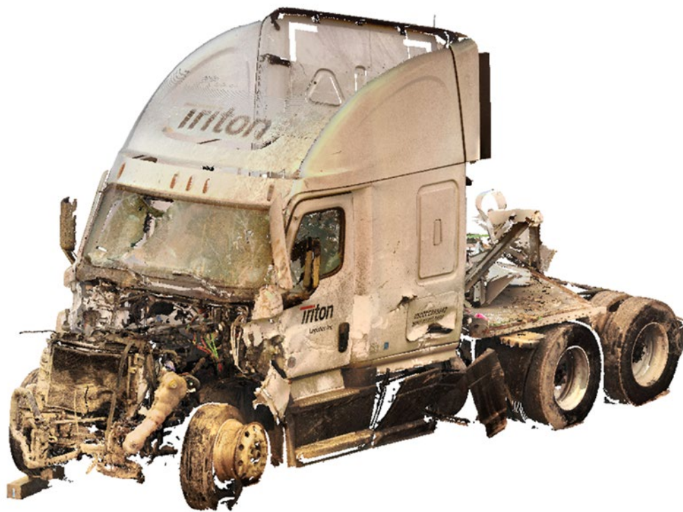
Figure 8: Screen capture depicting an oblique view of the Freightliner truck tractor 3D point cloud.
