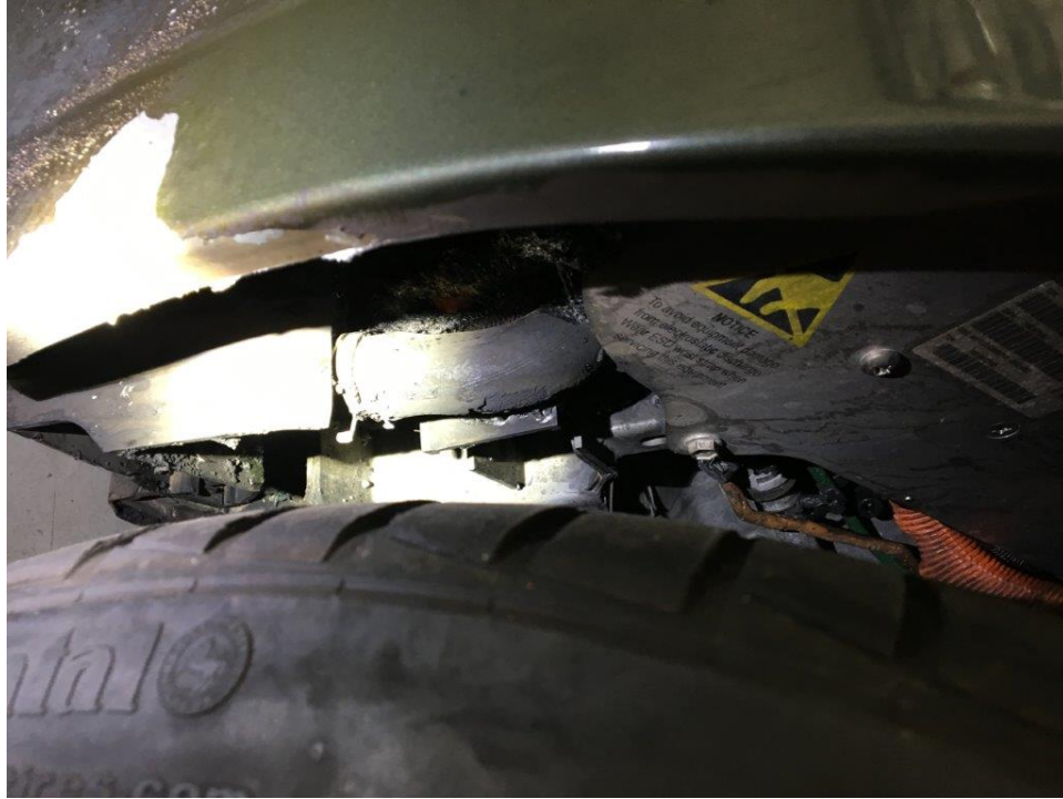
Burbank Inspection Photo 11: Left Front Wheel Well Access with portions of inner fender removed
