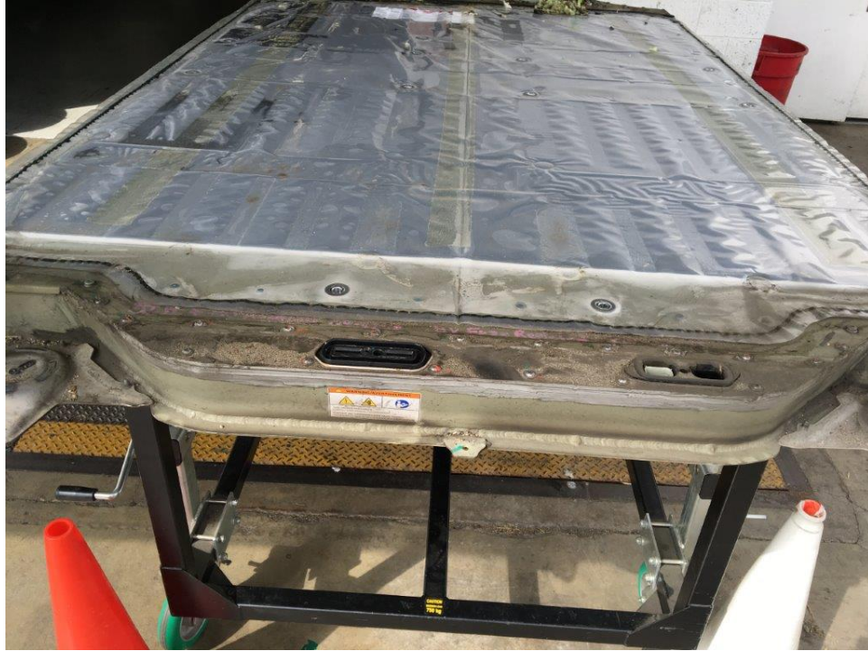
Burbank Inspection Photo 23: battery pack as removed, aft looking forward
