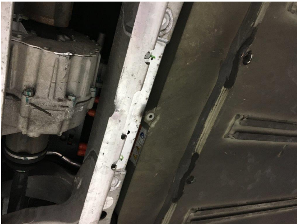
Burbank Inspection Photo 18: damage to rear motor and deflector
