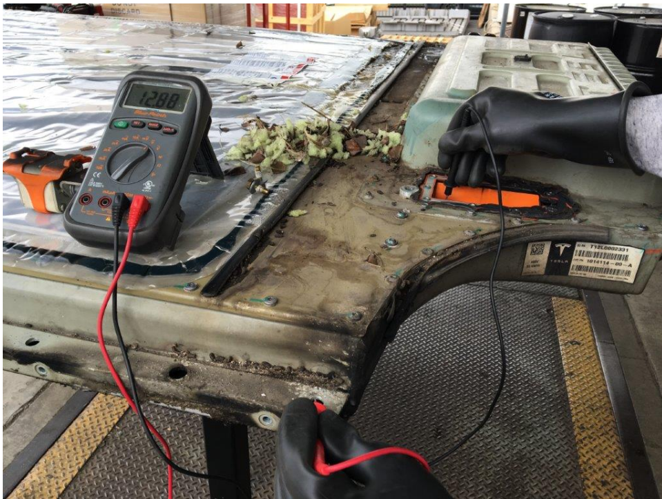
Burbank Inspection Photo 36: view showing voltage test to aft terminal of battery case
