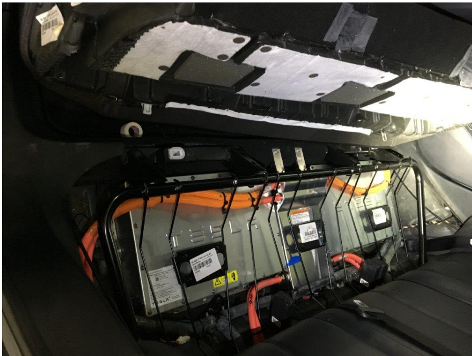
Burbank Inspection Photo 22: interior back, seat flipped up to see battery access
