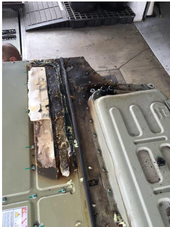
Burbank Inspection Photo 34: left front battery pack, showing thermal damage
