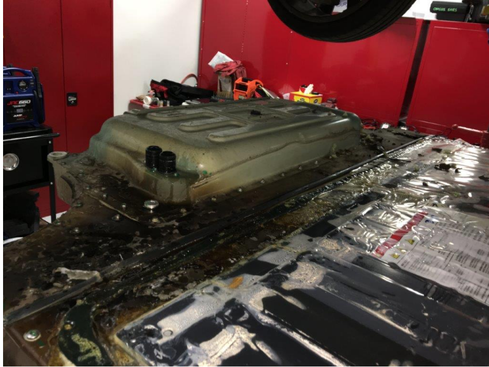
Burbank Inspection Photo 25: left front pack as dropped from vehicle
