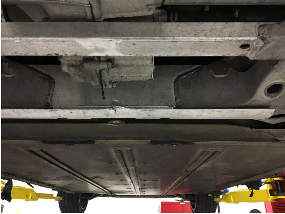
Burbank Inspection Photo 17: damage to rear motor and deflector overall
