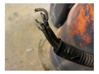
While we were unable to inspect the generator or the terminal box at the exact time of failure, it's our understanding that this harness is what was laying across the terminal posts, causing the arc'ing between terminals and ultimately, the generator to shut down.
