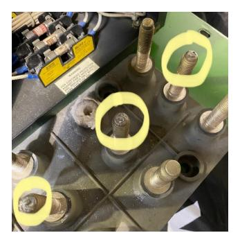
The harness that is present inside this terminal box was found to be blown completely in half. Pictured below, this is how it was received into our facility:
