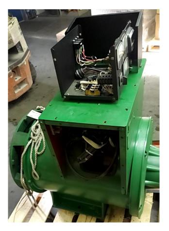
Once this repaired generator leaves our facility, the top cover (where the black control panel rests) must be removed in order to make internal connections to wire and install the generator on the vessel. If the personnel installing or wiring this generator is not careful to then replace the harness as it was, it could potentially lay across the terminal block which is what we believed happened to cause this failure.
