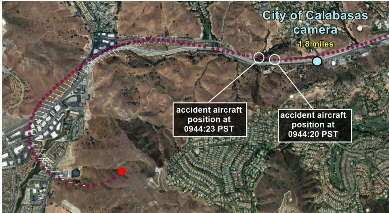
Figure 19 – City of Calabasas west-facing camera location. Yellow text identifies approximate distance from cameras to accident location. Accident location denoted by the red circle. The accident aircraft's ADS-B flight track is plotted by the purple circles/line with aircraft positions matching timestamps in Figures 20 and 21 identified.
