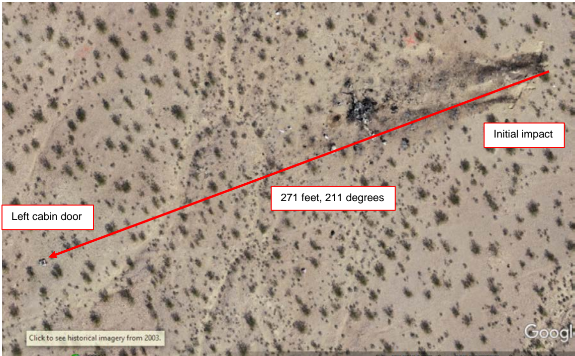
Figure 6 – Excerpt from Google Earth orthomosaic from initial impact to left cabin door.
