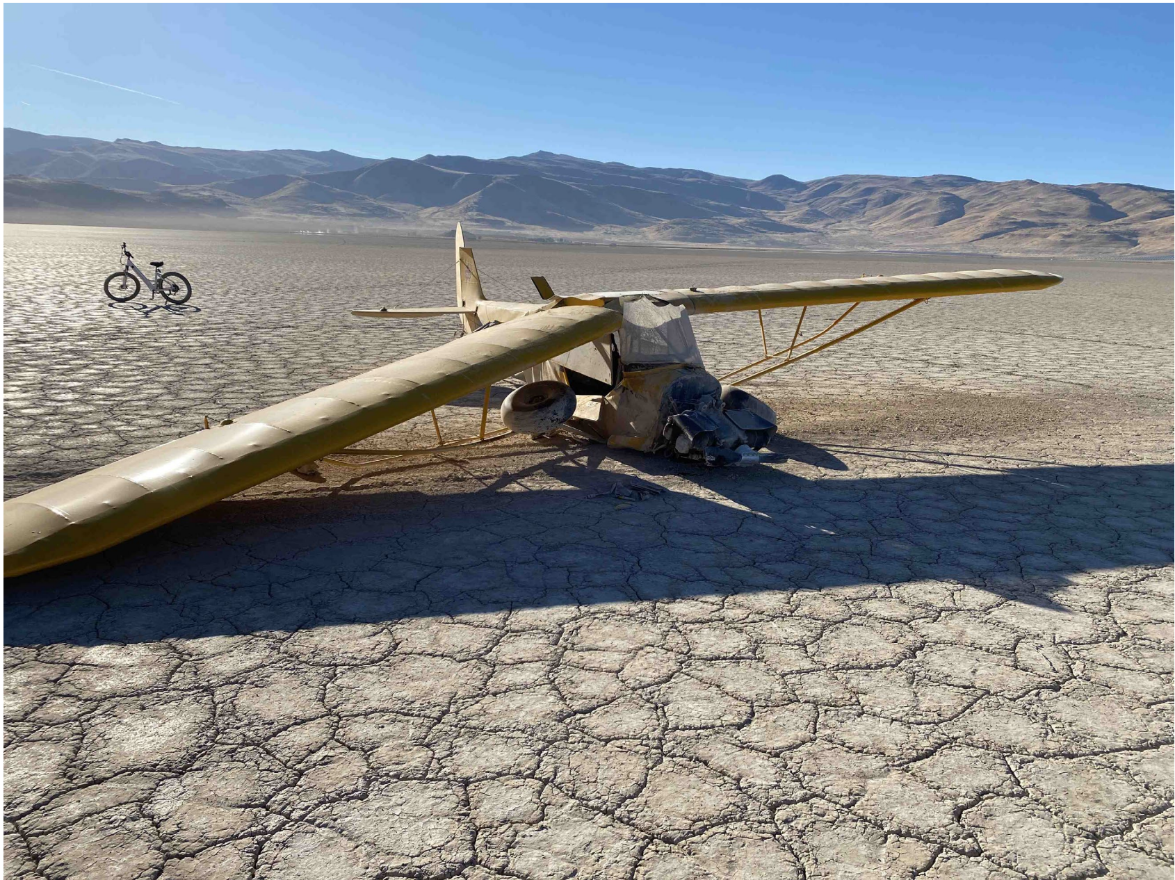
Photo 1 – Forward right view of airplane damage (Photo courtesy of FAA)
