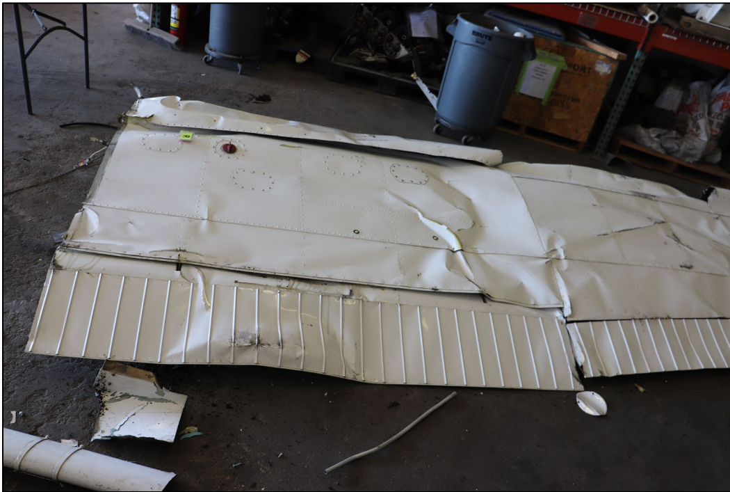
Figure 3: View of right wing damage.
