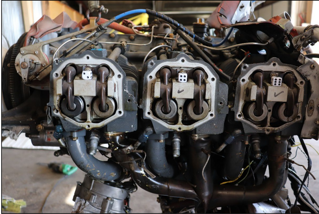
Figure 6: View of left side of the engine with the rocker box covers removed.
