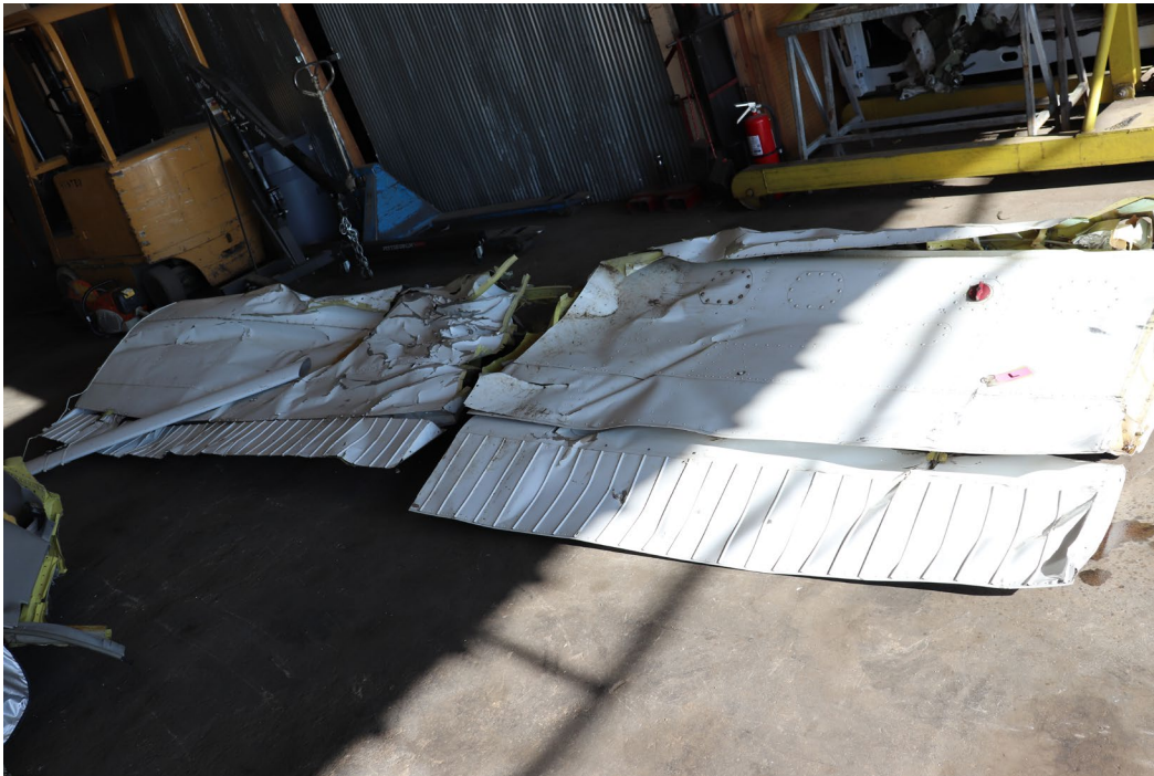
Figure 2: View of left wing damage.
