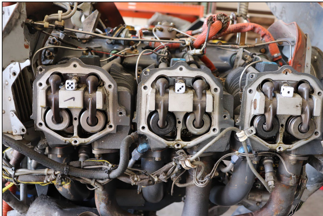
Figure 7: View of right side of the engine with the rocker box covers removed.
