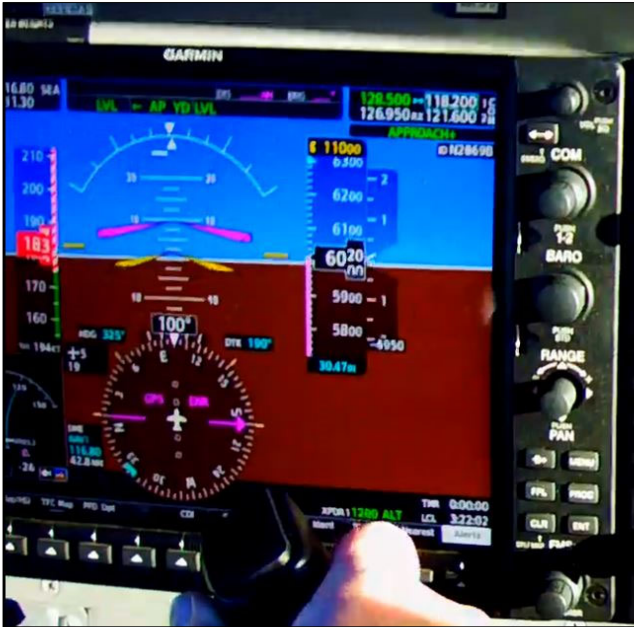
Figure 20. Video frame from Flight 07 showing an airspeed of 183 KIAS, 8 knots above V_{MO} .
