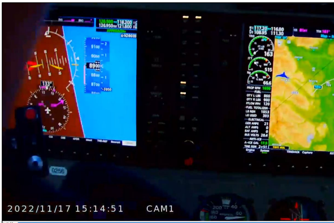
Figure 17b. Video frame from Flight 07 condition 5.6L, showing a roll angle past -60° following the stall break. The PFD was obscured by the pilot's body for a few seconds after the stall, but recorded data indicates that the roll angle reached -83°. Subsequent frames show the pitch angle at about -45°.
