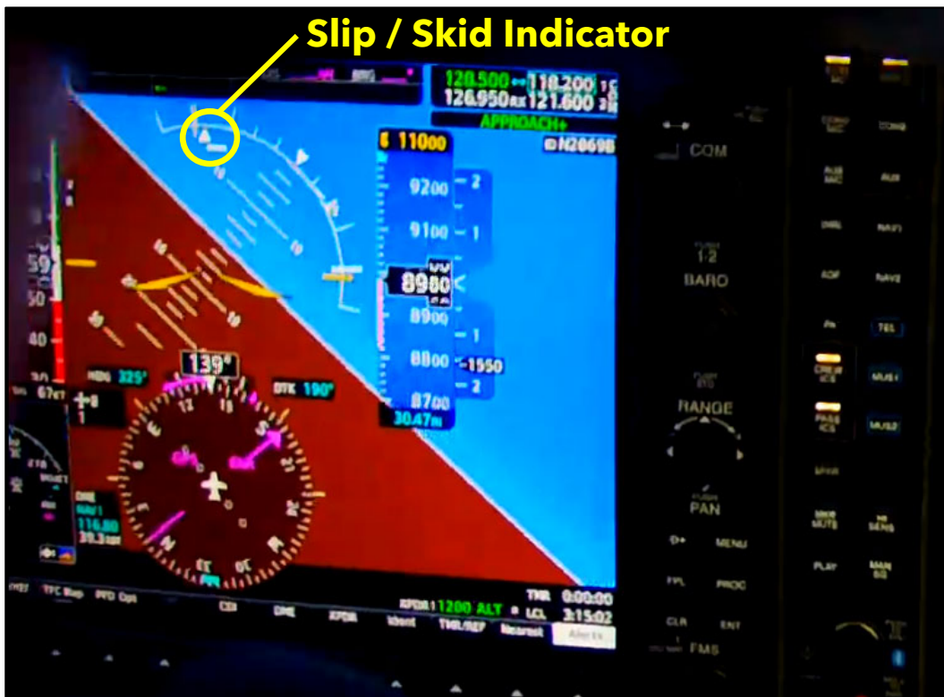
Figure 17a. Video frame from Flight 07 condition 5.6L, showing displacement of the Slip / Skid Indicator bar, and a roll angle greater than 30° just prior to the stall break.
