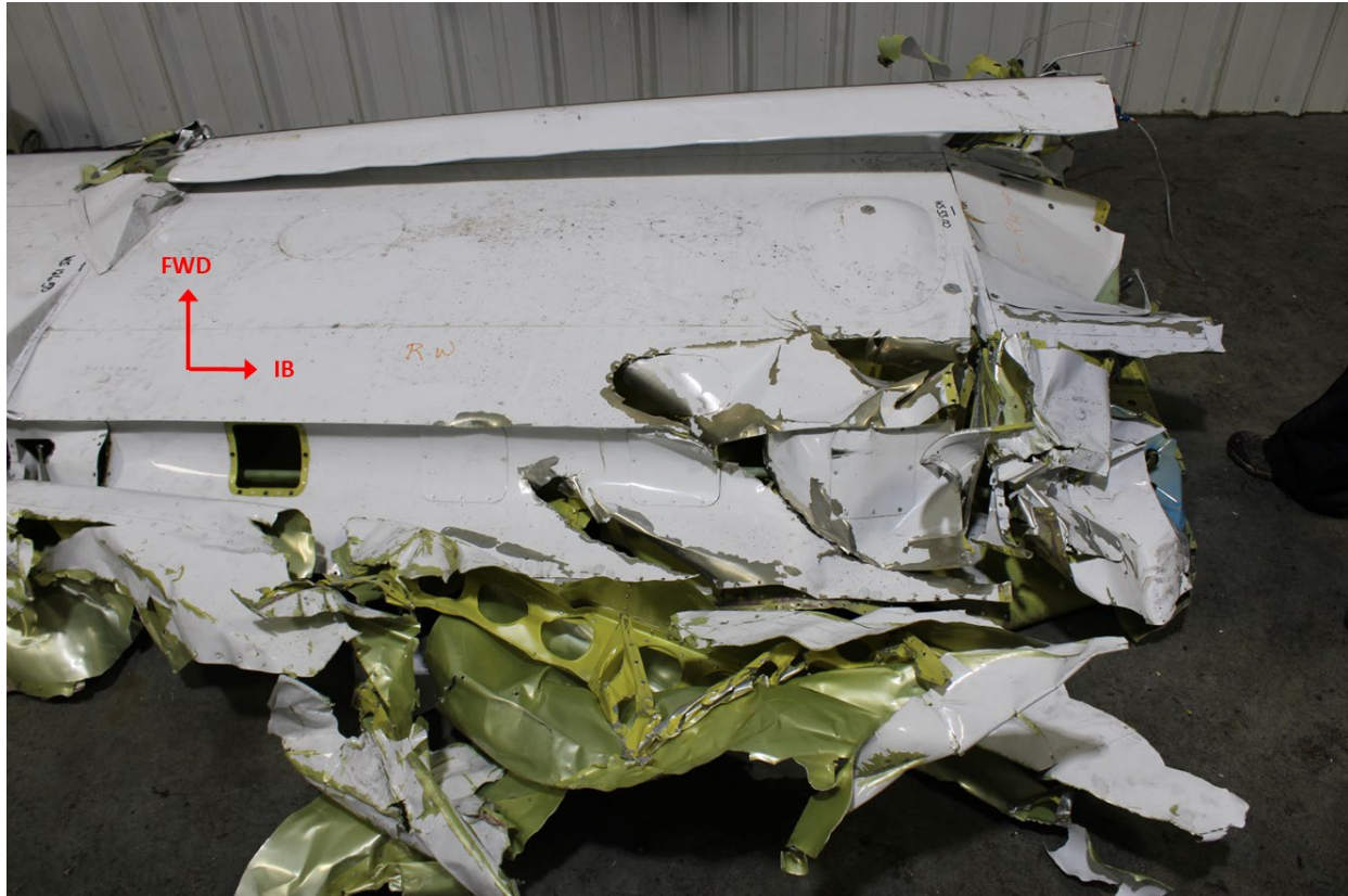
Figure 6. Right wing lower surface diagonal cuts WS 35-84 (NTSB photo)
