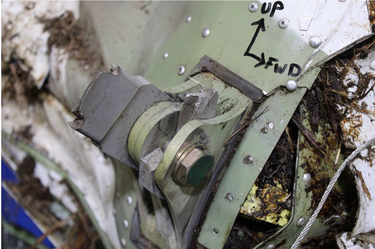
Figure 8. Fractured right strut lower fittings in fuselage clevis (NTSB photo)
