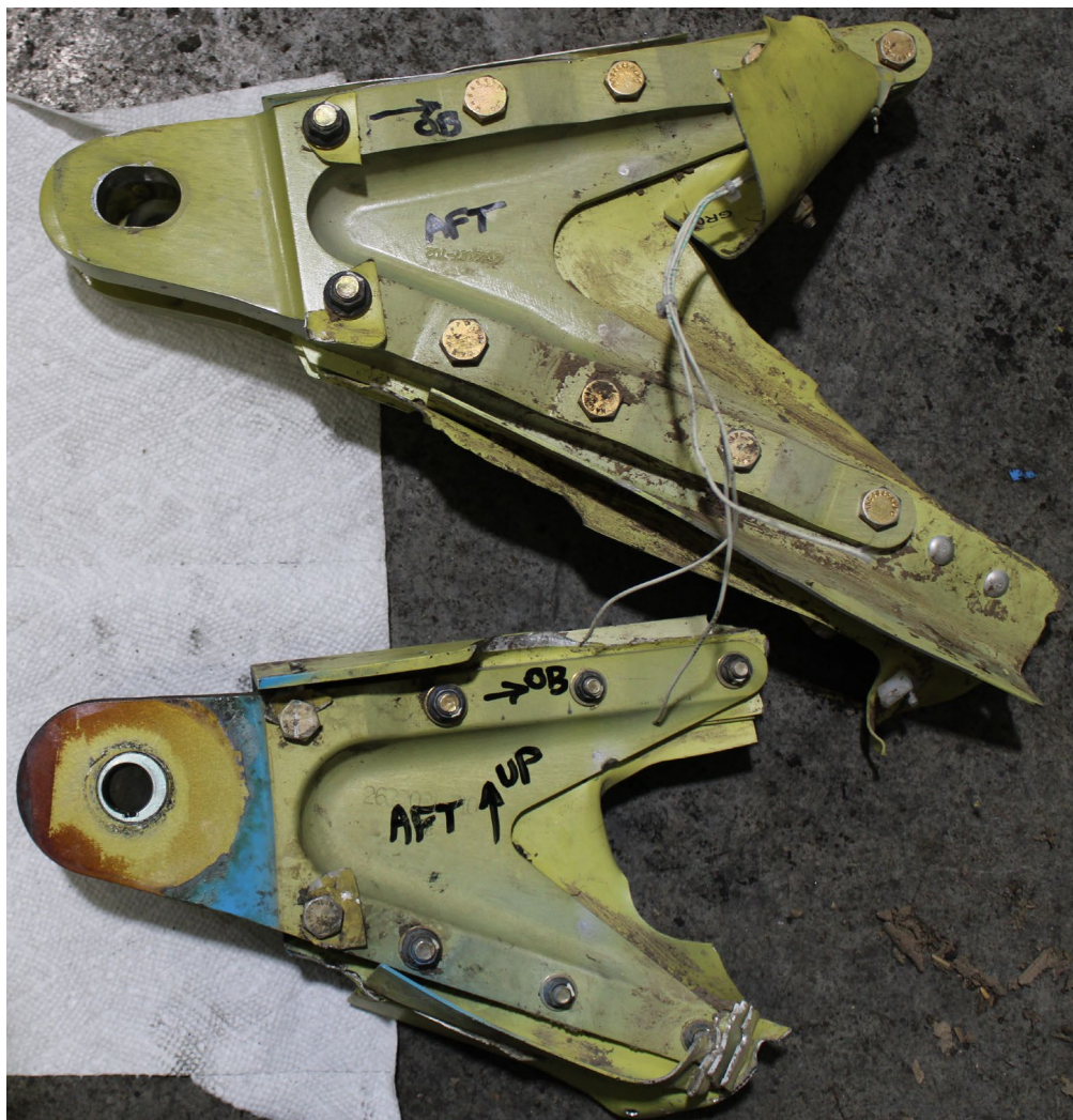
Figure 9. Right wing forward and aft spar attach fittings, aft side, after disassembly (NTSB photo)
