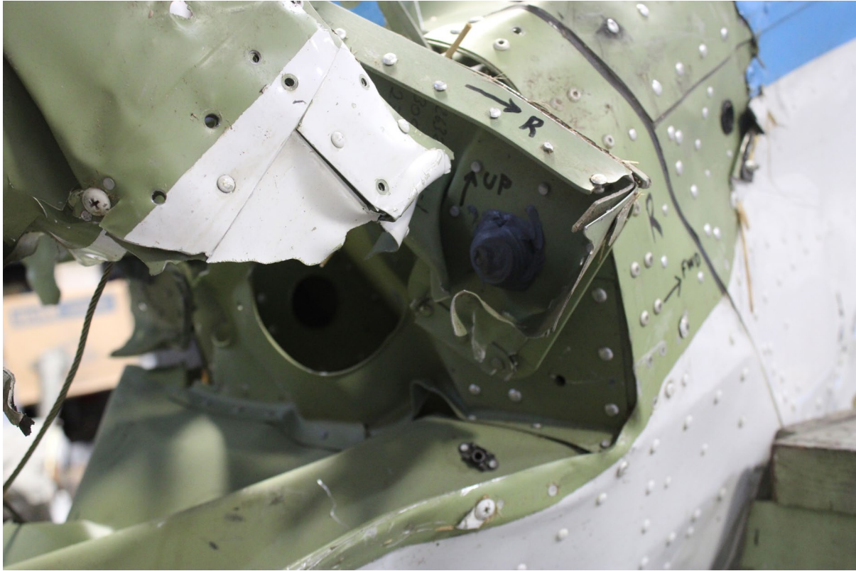
Figure 3. Horizontal stabilizer forward spar right attach point, looking forward (NTSB photo)
