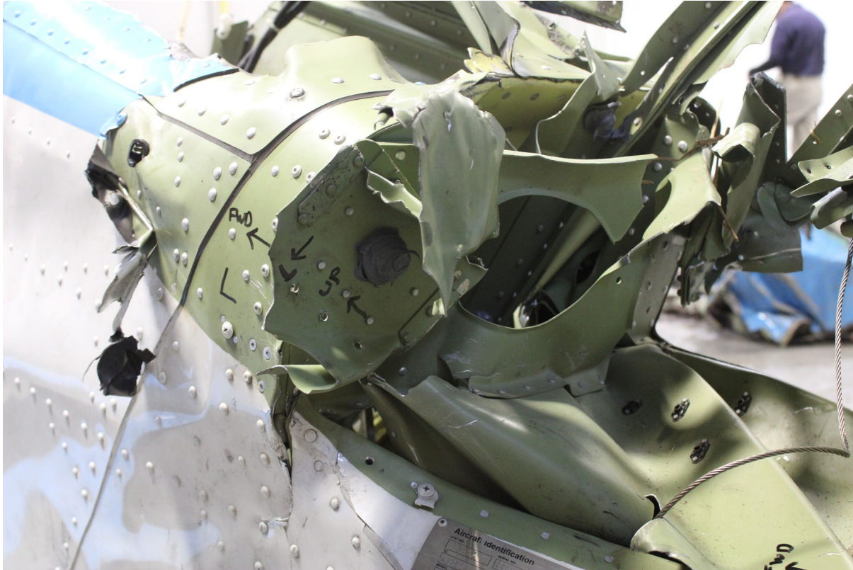
Figure 4. Horizontal stabilizer forward spar left attach point, looking forward (NTSB photo)
