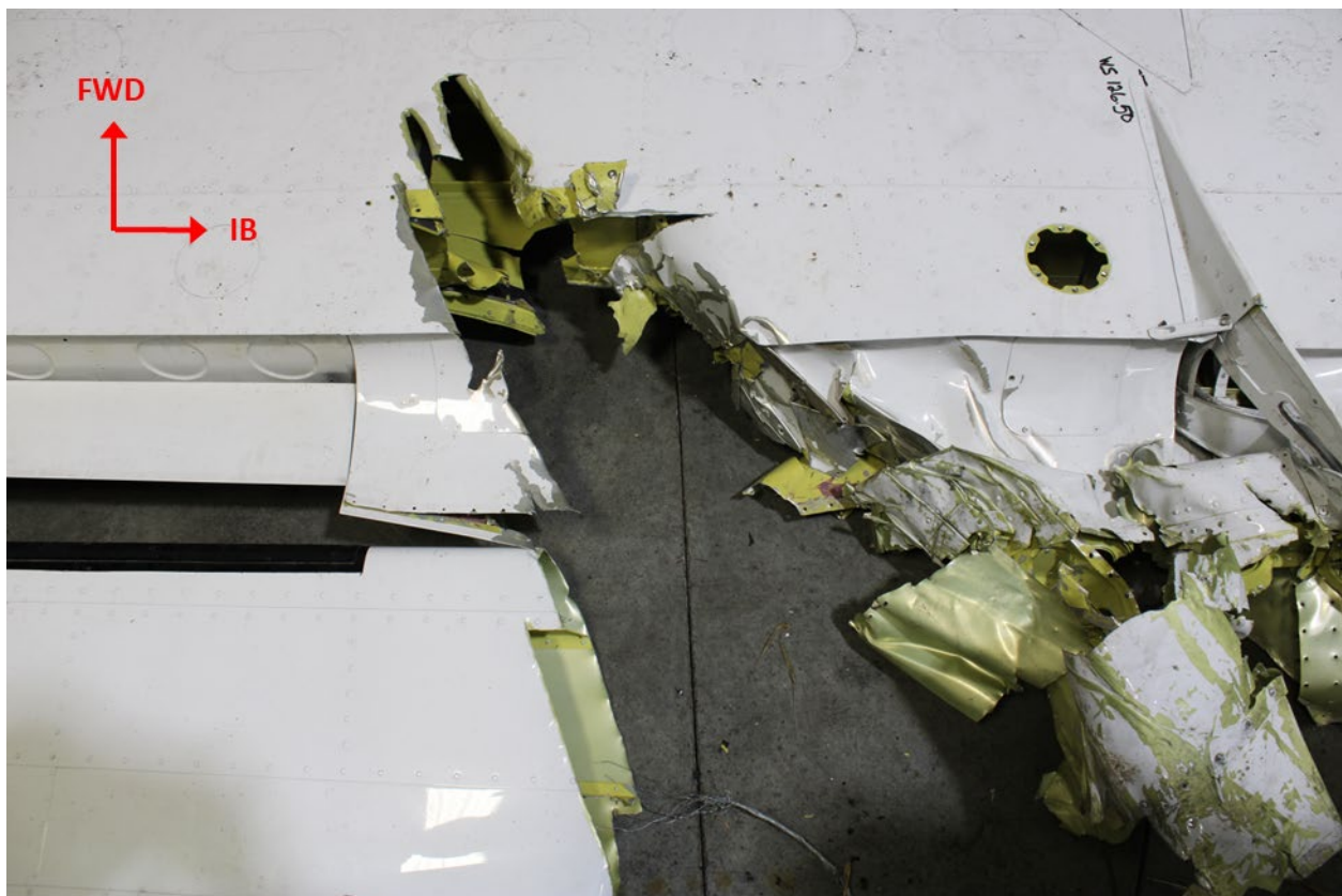
Figure 5. Right wing lower surface diagonal cuts WS 141-170 (NTSB photo)
