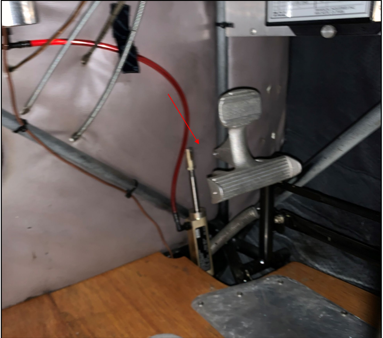
Figure 1: View of right pedal disconnected from the brake cylinder.
