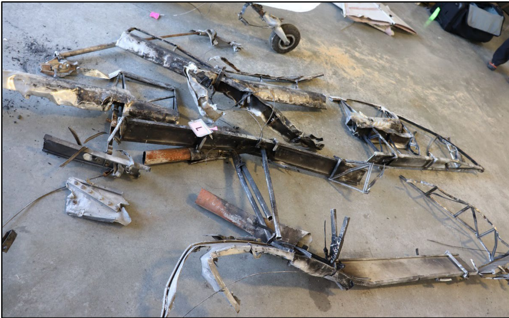
Figure 3: View of left wing thermal damage.
