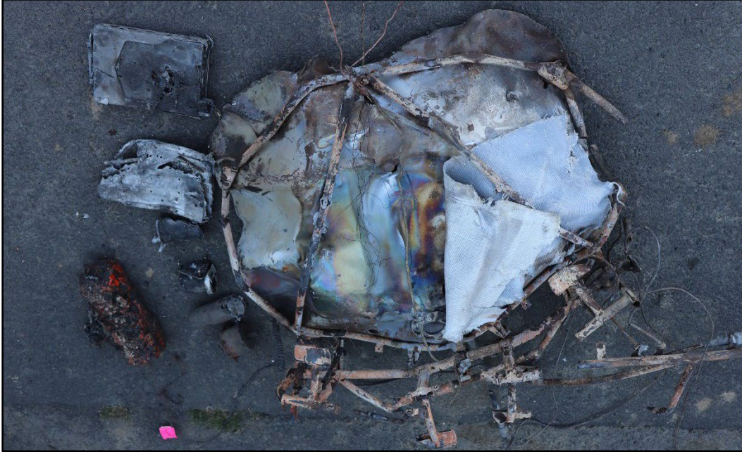
Figure 1: View of airplane cockpit area with impact and thermal damage.
