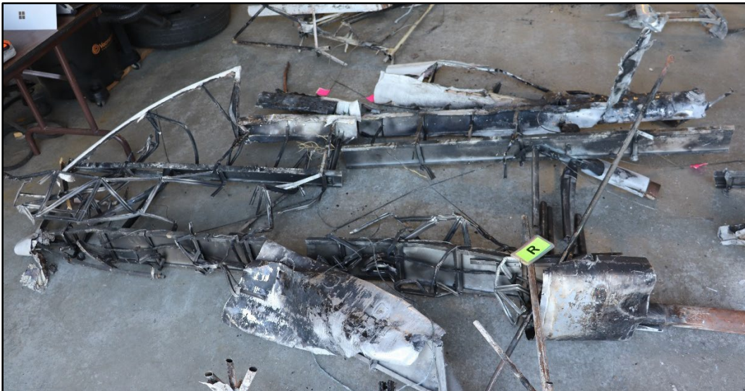
Figure 2: View of right wing thermal damage.
