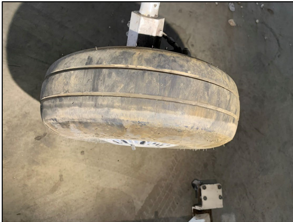
Figure 3: Main Landing Gear Tire as viewed from the top side (note markings on outer edge).
