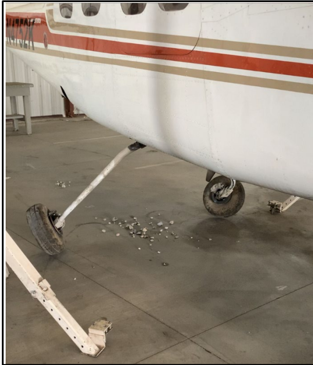
Figure 2: Main Landing Gear in transient for extension (note outer edge of tire).
