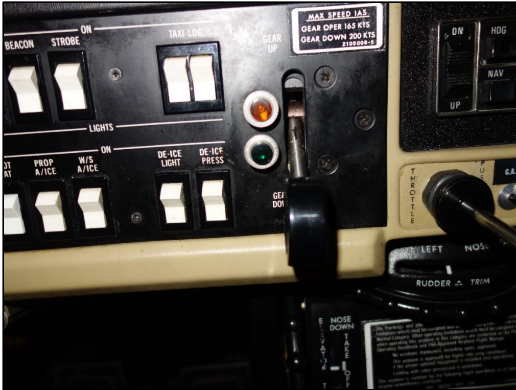
Figure 1: Land Gear Lever and Landing Gear Position Indicator Lights.
