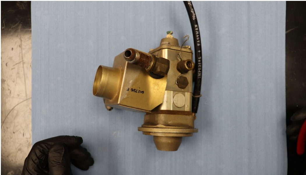
Figure 1: View of fuel pump during exam (photo courtesy of the NTSB)
